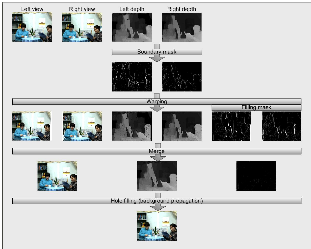
Figure 28: Flow diagram for VSRS 1D mode.
