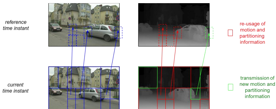
Figure 20: Illustration of the concept of motion parameter inheritance.
