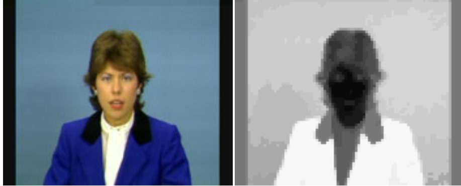
Fig. 6. The original frame from the test video sequence CLAIRE (left image) and its scalar chrominance image (right).
