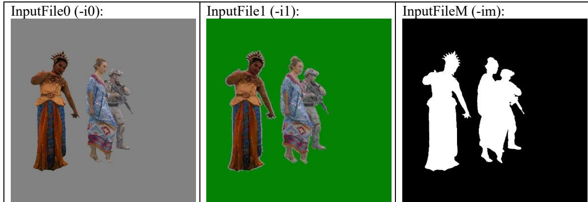
In an example above, the IV-PSNR value is calculated only for occupied pixels (as indicated by mask), so different color of the unoccupied background does not impact outputted quality.
