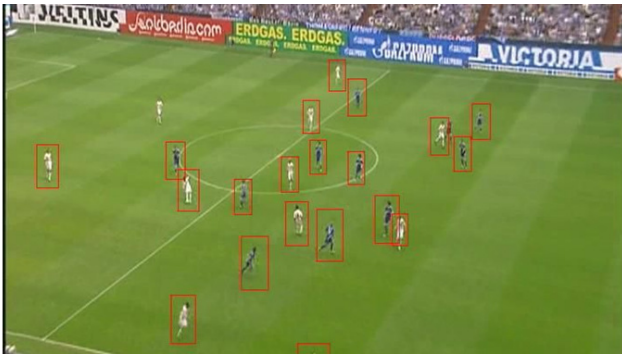
Fig. 12. A result of a player detection (HOG-PCA classification).
