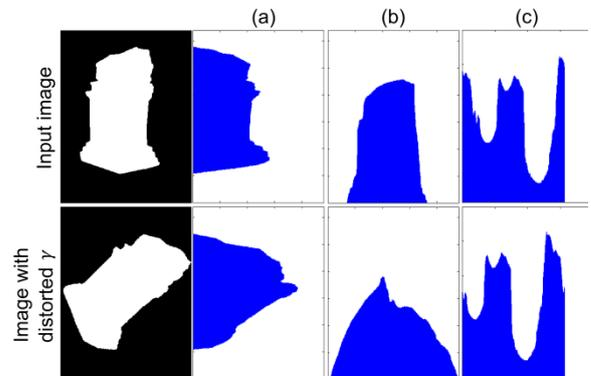
Figure 3. Visualization of histogram shape variation due to the  $\gamma$  rotation of  $i$ -th input image. (a) – vertical histograms, (b) – horizontal histograms, (c) – radial histograms depicted as a function  $Distance(\text{angle}[rad])$ .
