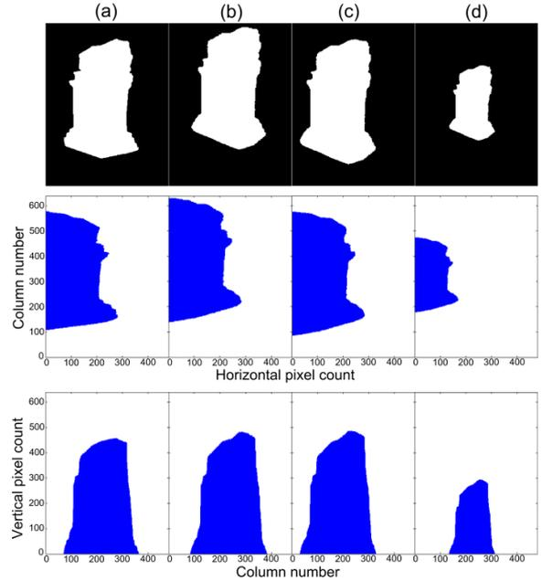
Figure 2. Visualization of known distortion of certain camera parameters. In columns: (a) – input image, (b) – reprojection with distorted  $\alpha$ , (c) – reprojection with distorted  $\beta$ , (d) – reprojection with distorted  $f$ .
