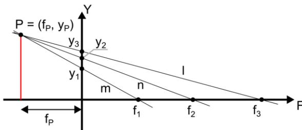
Figure 4. Visualization of 3 reprojection lines  $m, n, l$  that cast the point  $P$  into image plane with respect to 3 focal lengths  $f_1, f_2, f_3$ . Visualization of system of equations to calculate corrected focal length  $f_3$ .
