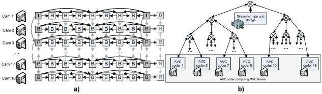
Figure 8. The MVC coding scheme (a) and the assessed model of the MVC coder (b)
