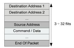
Figure 6. The NoMC packet format
