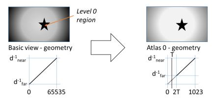
Figure 15: When the source material has invalid geometry values, the geometry coder not only performs u(16) to u(10) scaling, but it also sets the geometry threshold to a configurated value (T) and the normalized disparity range is modified such that value 2T corresponds to the far geometry.
