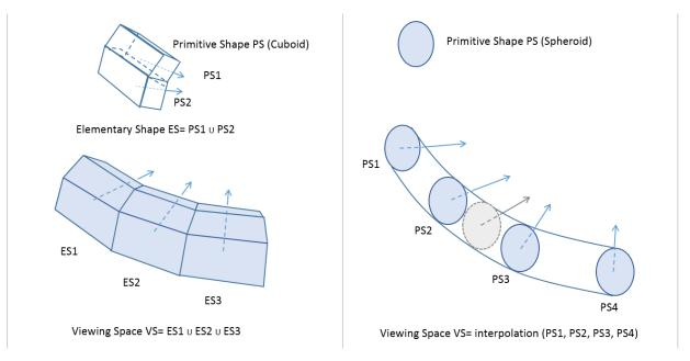
Figure 24: Illustration of VS creation with additive CSG (left) and interpolation (right).
