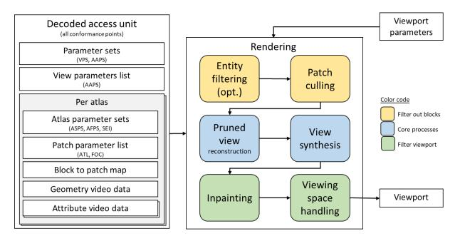
Figure 17: Process flow for the TMIV renderer.
