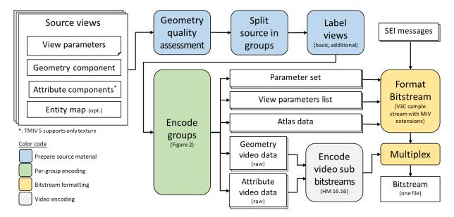
Figure 1: Top-level diagram of the TMIV group-based encoder.
