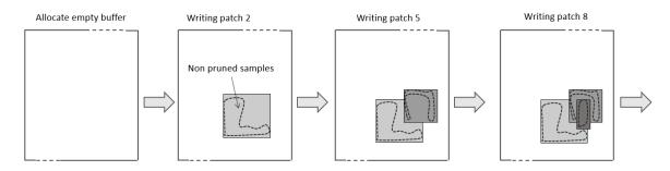
Figure 13: Successive writing of patches into an atlas.
