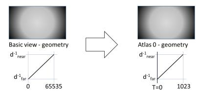
Figure 14: When the source material has only valid geometry values, the geometry coder only performs u(16) to u(10) scaling and the geometry threshold is set to zero to signal full occupancy.
