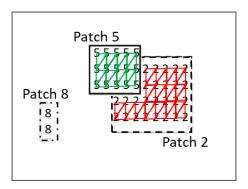
Figure 20: Creating a mesh from an atlas. Triangles between pixels from Patch 5 and 2 are omitted. Note that Patch 8 is not drawn because no triangle can be formed. Unused pixels are skipped too.
