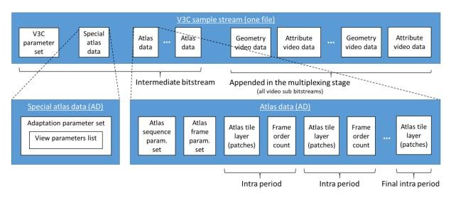
Figure 16: V3C sample stream with MIV extensions.
