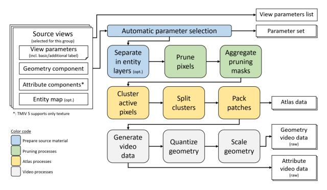
Figure 2: Top-level diagram of the TMIV single-group encoder.
