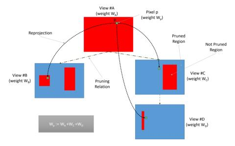
Figure 21: graph-based pruning: weight recovery procedure.
