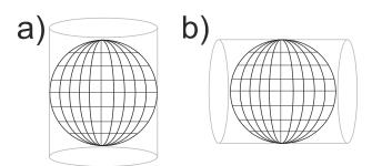
Figure 22: Cylinders used in the projection of a sphere on a flat image in a) equirectangular projection and b) transverse equirectangular projection.
