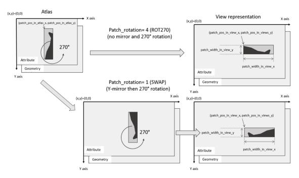
Figure 12: Meaning of patch related parameters.
