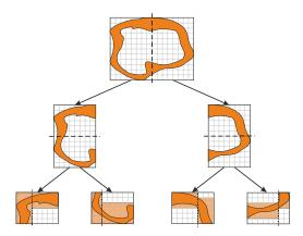
Figure 11: Recursive splitting of the cluster; dashed lines: C-splitting, dotted lines: L-splitting.
