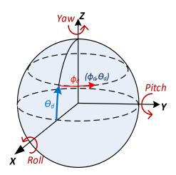
Figure 25: OMAF coordinate system illustrating the directions of positional and rotational units.
