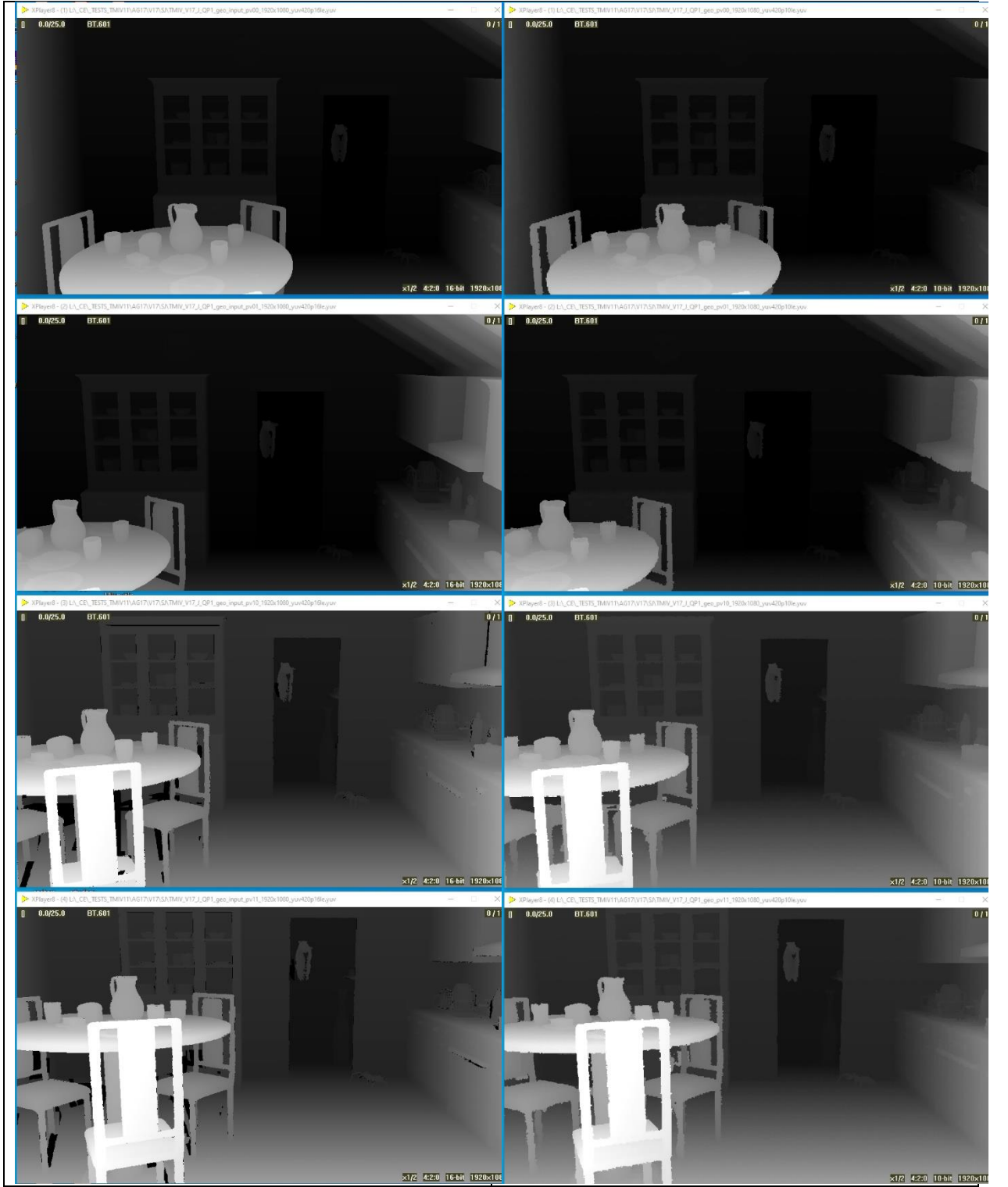
Fig. 6. Input depth maps (left) vs. output depth maps (right); fully occupied depth maps for views from 0 th atlas (1 st and 2 nd rows), and depth maps with holes for views from atlases 1 and 2 (3 rd and 4 th rows).
