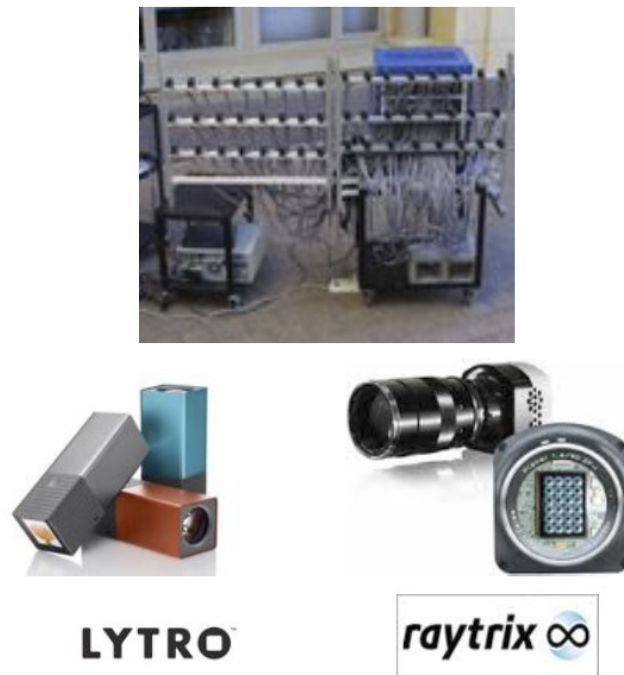
Fig. 1. Lightfield images acquisition systems.
