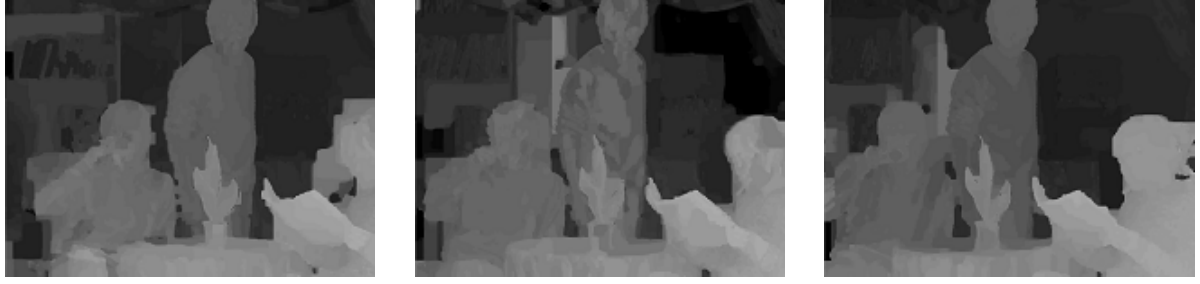
Figure 6.3.1 – Example of an inter-view depth map inconsistency in the sequence "Newspaper" [CFP]. The cameras are 02, 04 and 06, beginning from the left-hand image.
