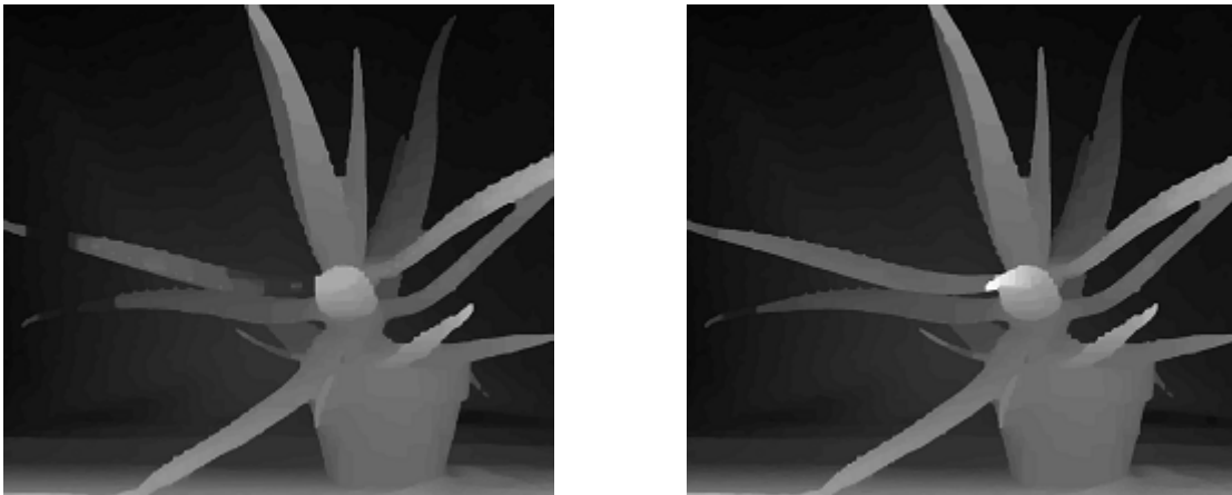
Figure 5.4.11. – Estimated depth map for camera 0. The depth map on the left was estimated with the original cross cost function while the right depth map was estimated using the proposed image edge incorporation technique.
