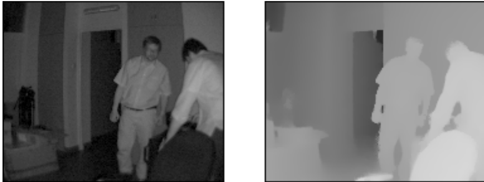
Figure 3.4.10 – Example intensity image and filtered distance map.
