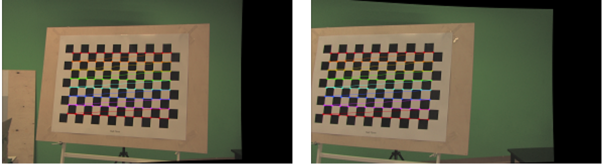
Figure 2.5.6 – Rectification result using an original, unmodified camera distribution line.
