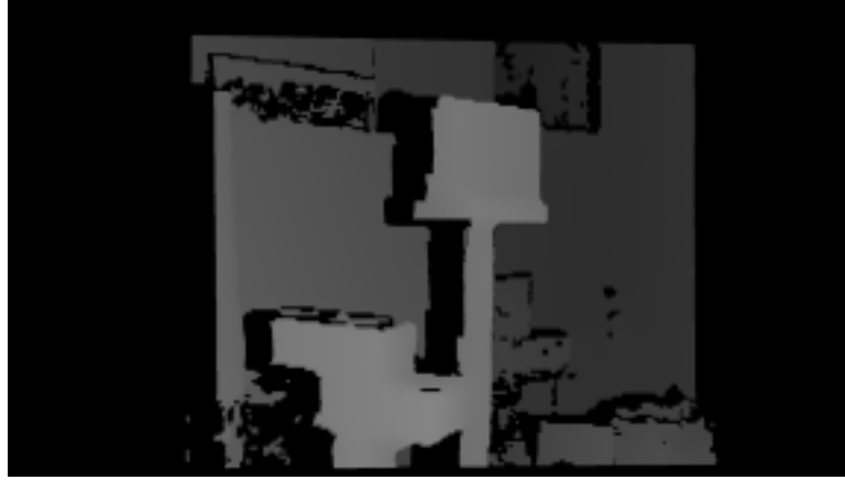
Figure 5.3.5 – Illustration of the rendered mesh of a 3D scene with disocclusion handling. The black colour indicates an unknown depth value.
