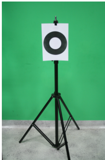
Figure 2.6.1 – Proposed marker used by the author for depth camera extrinsic parameter estimation.
