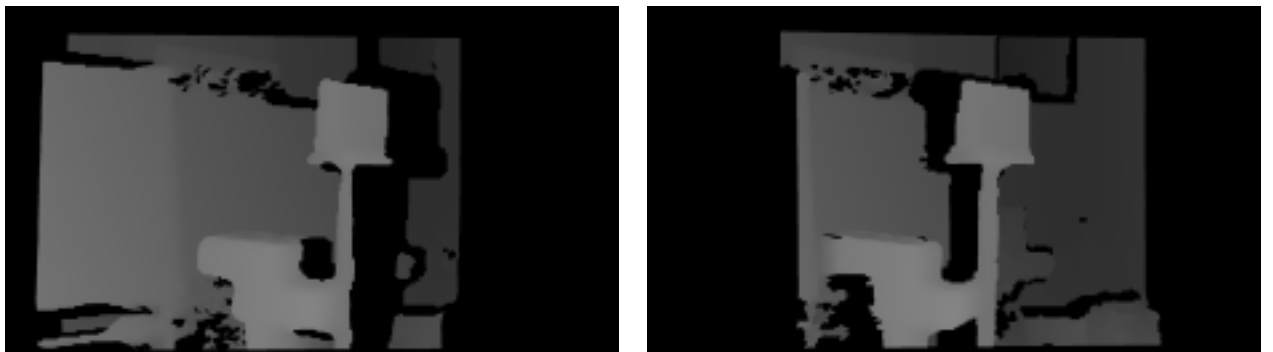
Figure 5.3.8. – Depth maps obtained using a single depth camera. Left image – the depth camera was located to the left of the video camera; right image – the depth camera was located to the right of the video camera.
