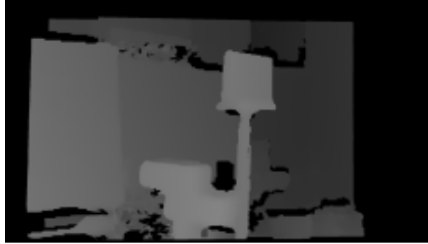
Figure 5.3.9. – Aggregated depth map which is the result of joining two depth maps that were obtained from individual depth cameras.
