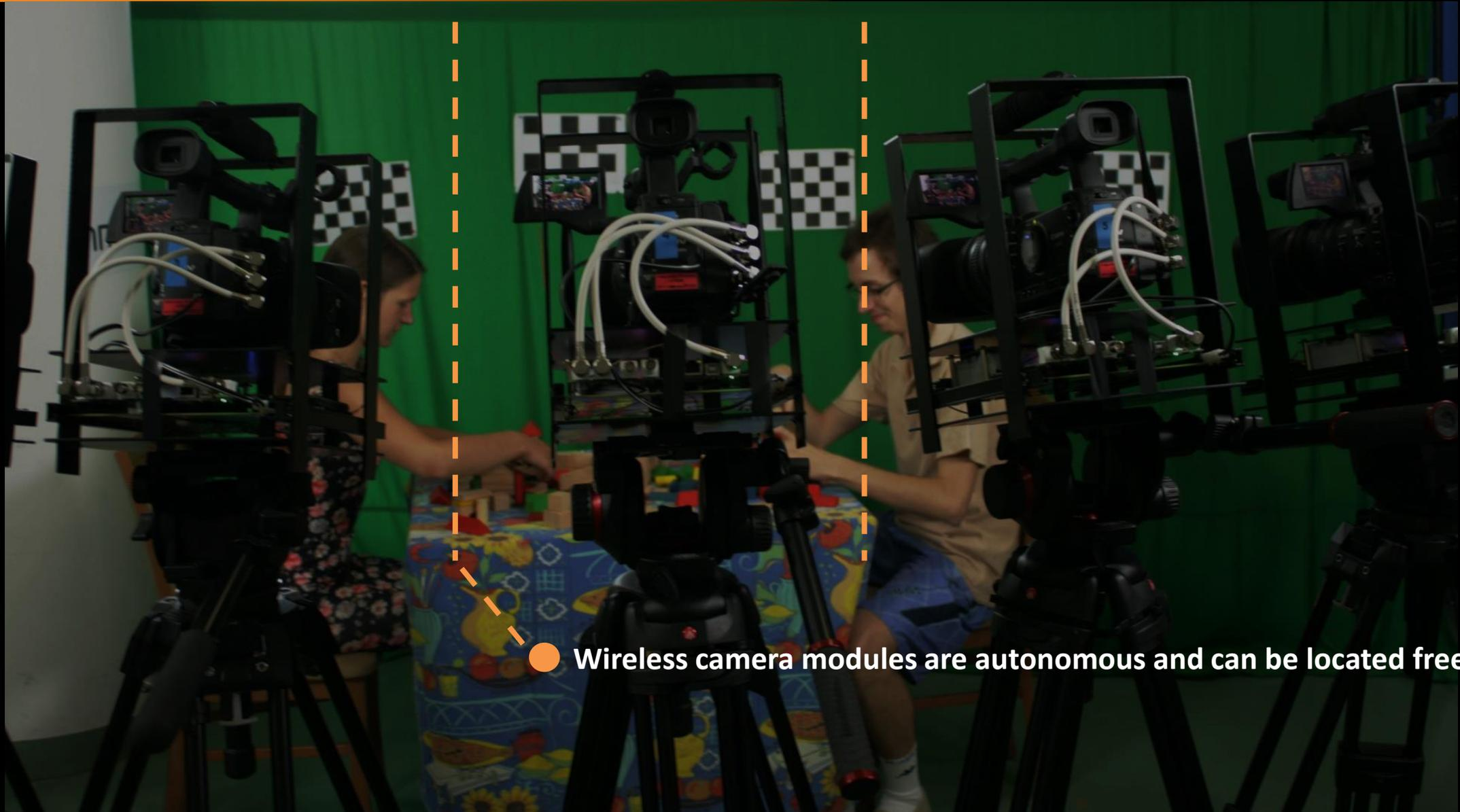
● Wireless camera modules are autonomous and can be located freely
