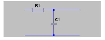
$\begin{array}{l} R1=4-20 \ k\Omega \\ C1=22-47 nF \end{array}$
