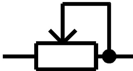
Figure 2.11 Potentiometer as a variable resistor
