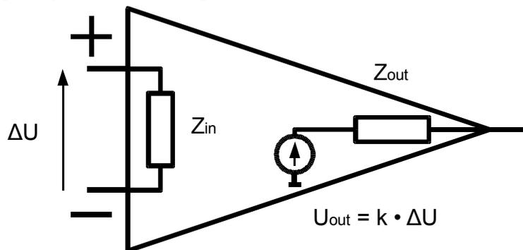
Figure 6.23 Input and output impedances of a real operational amplifier
