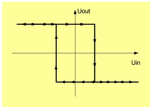
Figure 6.32 Inverting Schmitt trigger example operation curve
