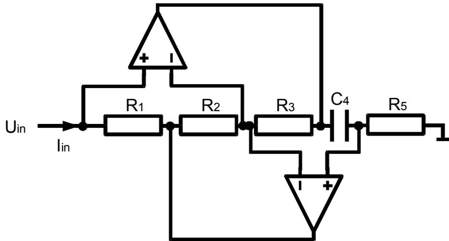
Figure 6.21 General impedance converter
