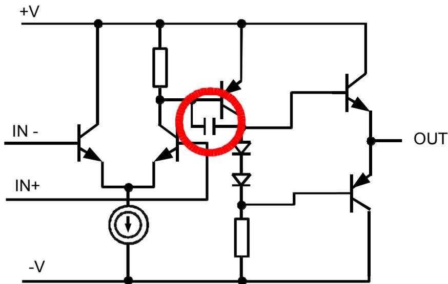
Figure 6.39 Frequency compensation of operational amplifier
