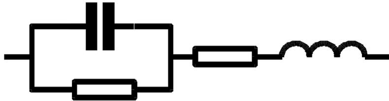
Figure 2.18 Model of parasitic elements of a real life capacitor
