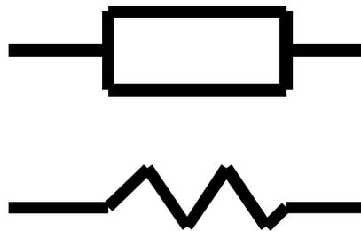
Figure 2.1 Schematic symbols for the resistor
