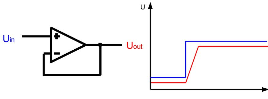
Figure 7.3 Operational amplifier output - slew rate limit. A slight offset of the signals is applied for clarity only.
