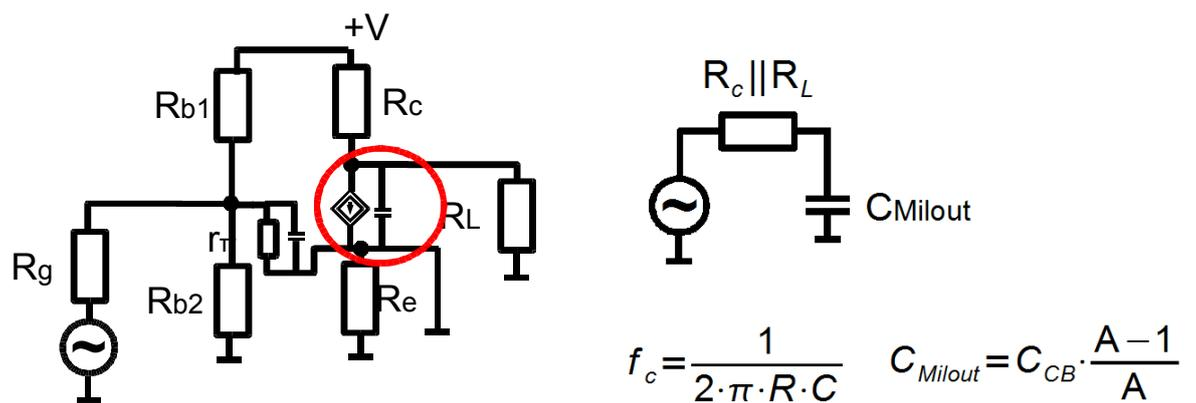
Figure 7.21 High frequency limit - collector side
