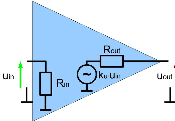
Figure 4.23 Basic amplifier model
