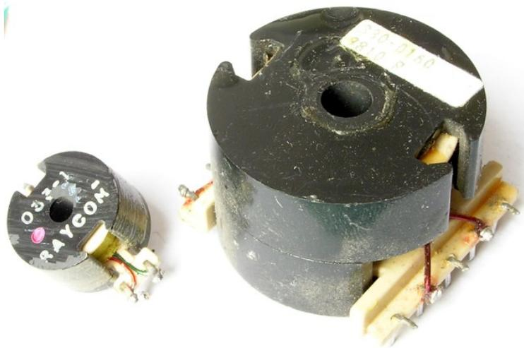
Figure 2.29 Small transformers example
