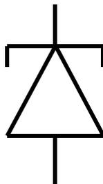
Figure 3.24 Tunnel diode symbol
