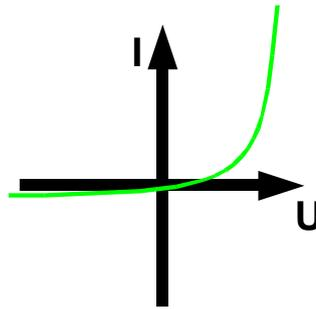
Figure 3.11 Diode model IV
