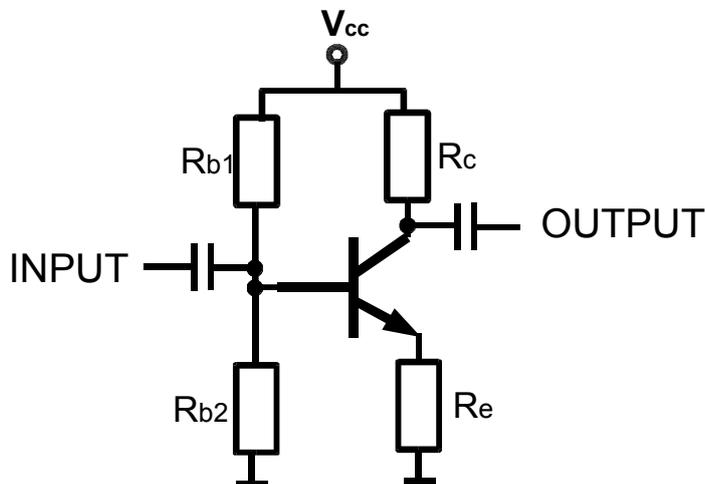
Figure 4.19 Typical single transistor amplifier
