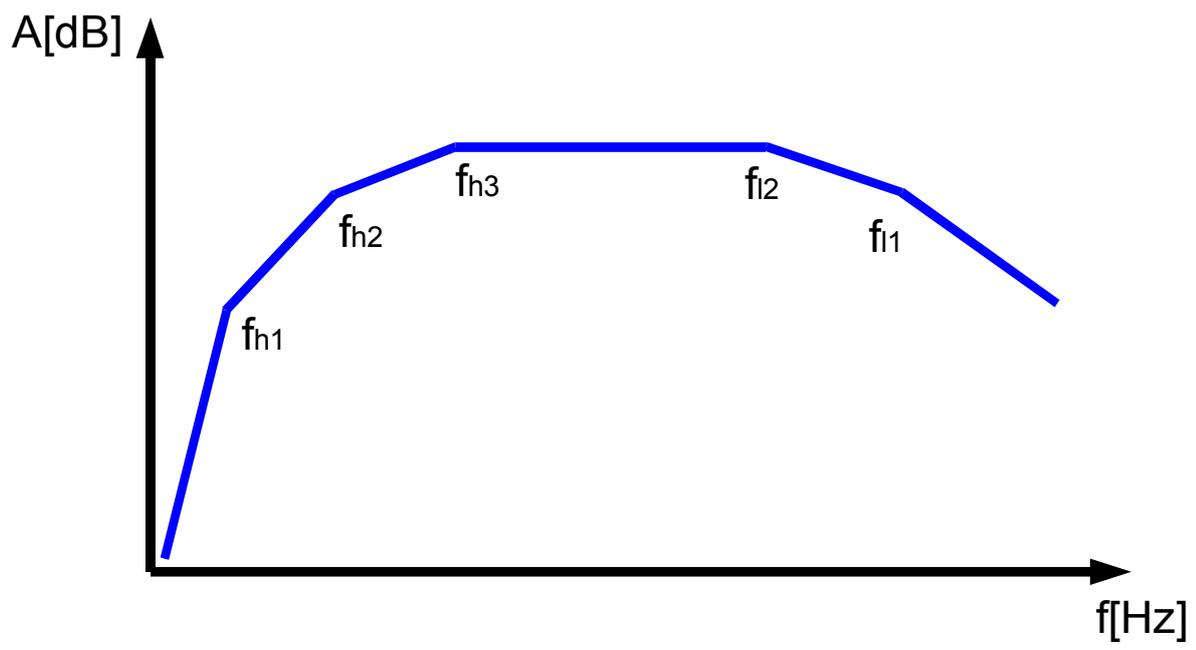
Figure 7.22 Frequency spectrum of a transistor amplifier
