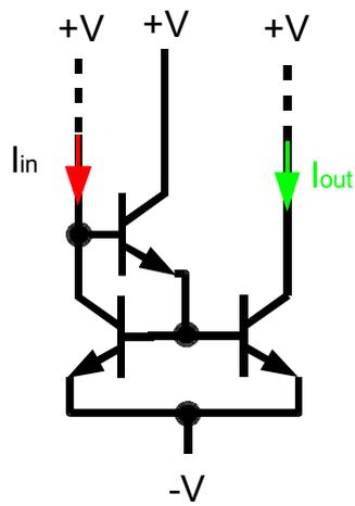
Figure 6.42 Current mirror with additional transistor improving symmetry
