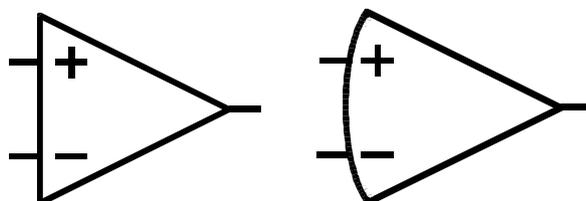
Figure 6.1 Operational amplifier - basic symbol
