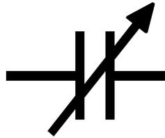
Figure 2.22 Variable capacitor symbol
