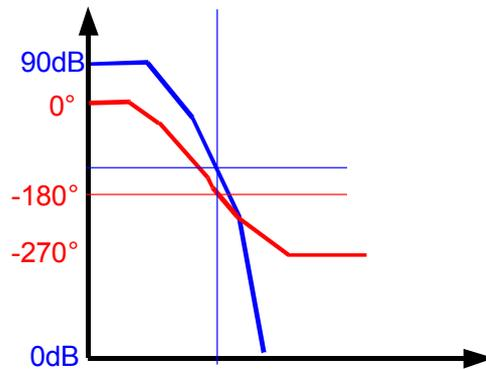
Figure 7.8 Uncompensated amplifier frequency response
