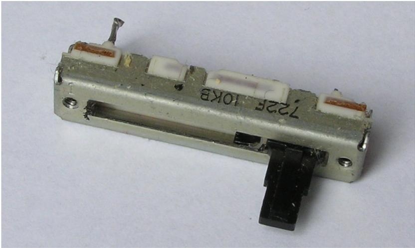
Figure 2.14 Slide potentiometer
