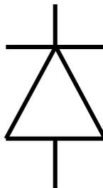
Figure 3.13 Rectifying diode
