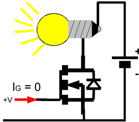
Figure 5.26 MOSFET working as a switch
