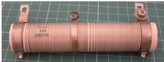
Figure 2.7 Wire wound resistor
