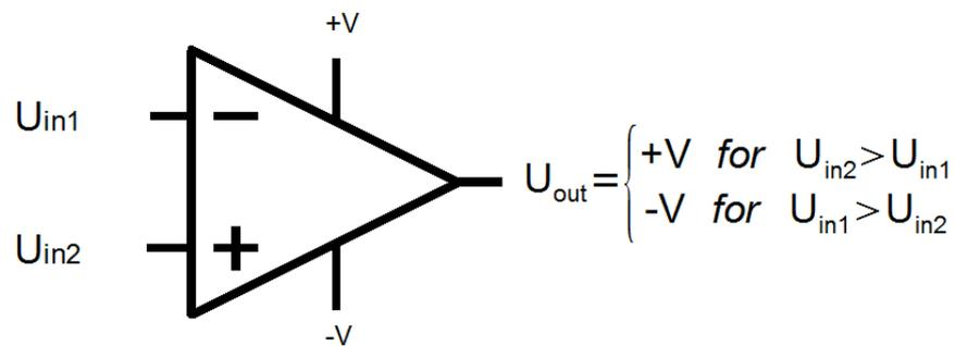
Figure 6.28 Comparator operation
