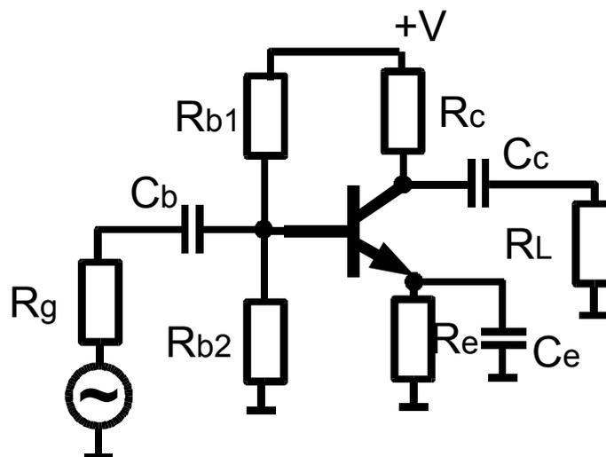
Figure 7.10 Transistor amplifier
