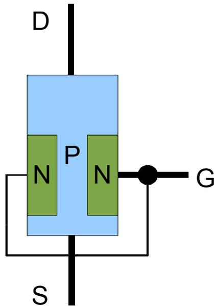
Figure 5.5 P channel JFET internal structure
