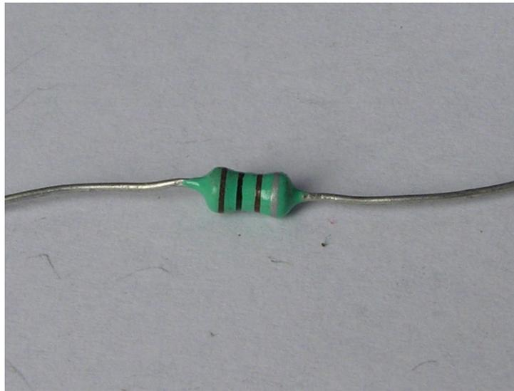
Figure 2.26 Small inductor example
