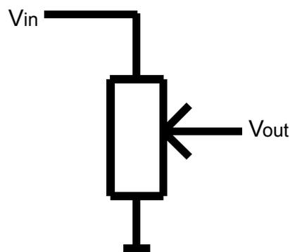
Figure 2.10 Potentiometer as a voltage divider
