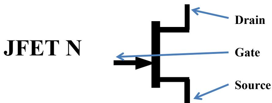
Figure 5.1 JFET-N transistor
