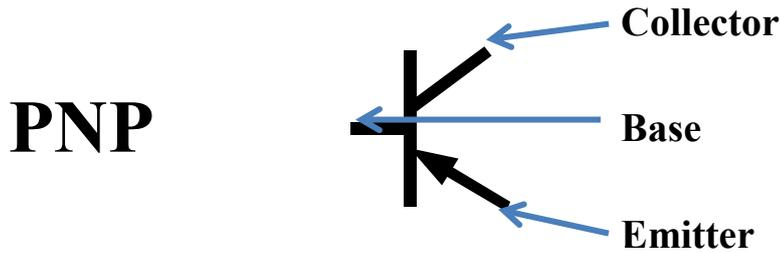
Figure 4.2 PNP transistor symbol
