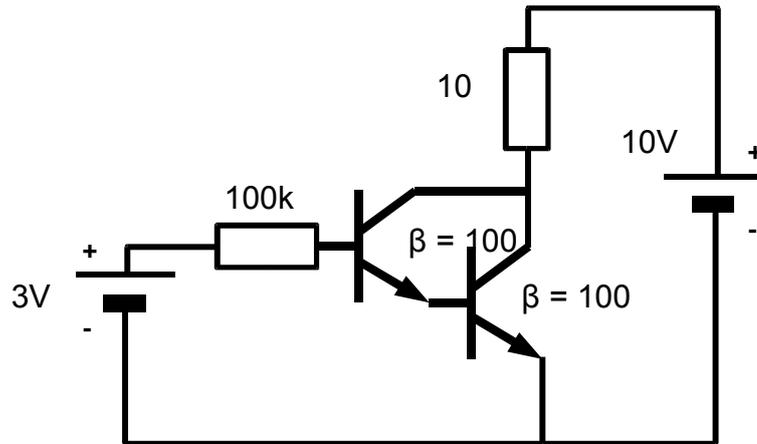
Figure 4.25 Two bipolar transistors connected together
