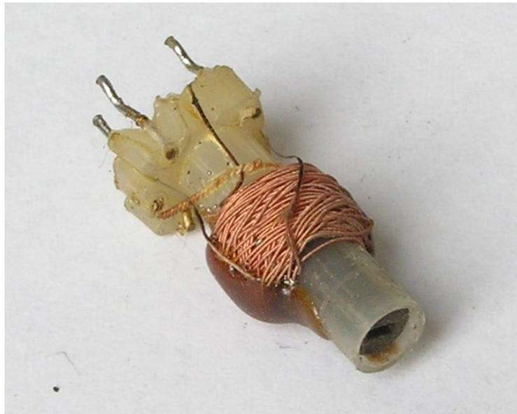
Figure 2.32 Variable inductor with screwed-in core
