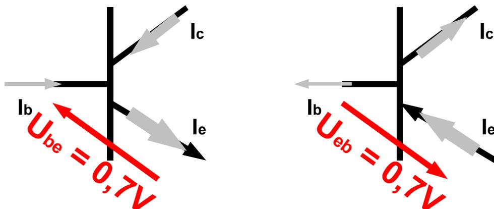
Figure 4.6 Polarization voltage for bipolar transistors NPN on the left, PNP on the right
