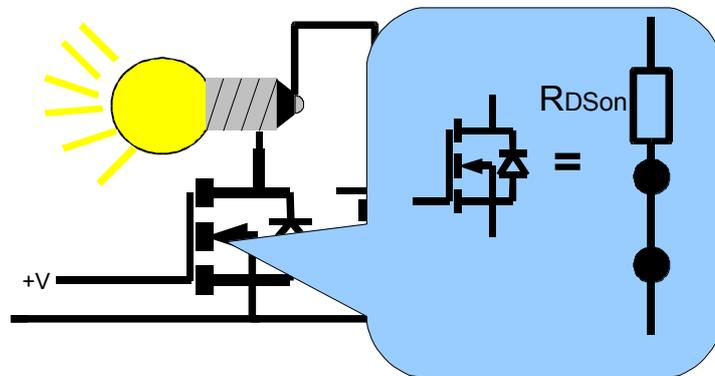
Figure 5.27 MOSFET as a switch - fully on
