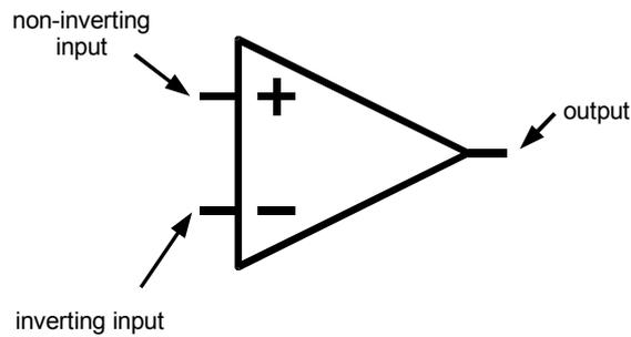
Figure 6.2 Operational amplifier terminals
