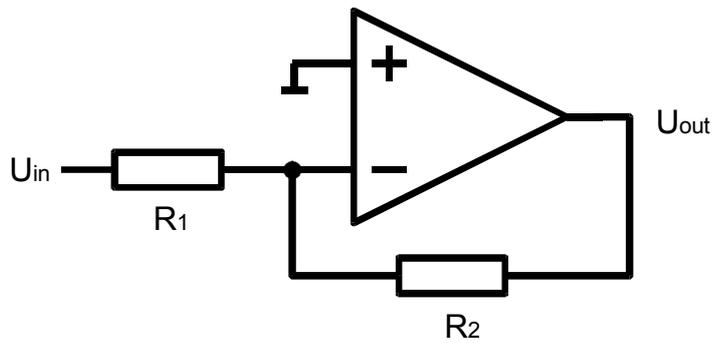
Figure 6.5 Inverting amplifier
