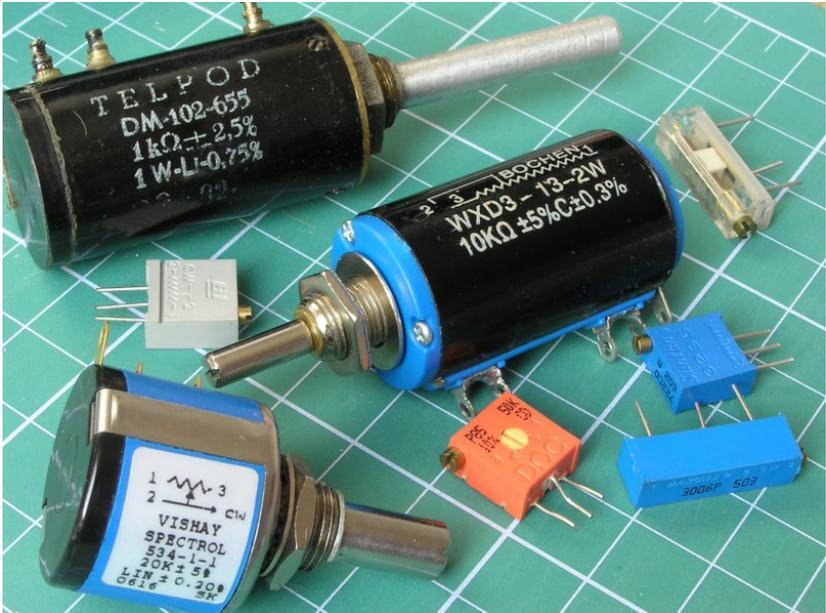
Figure 2.13 Multi-turn potentiometers
