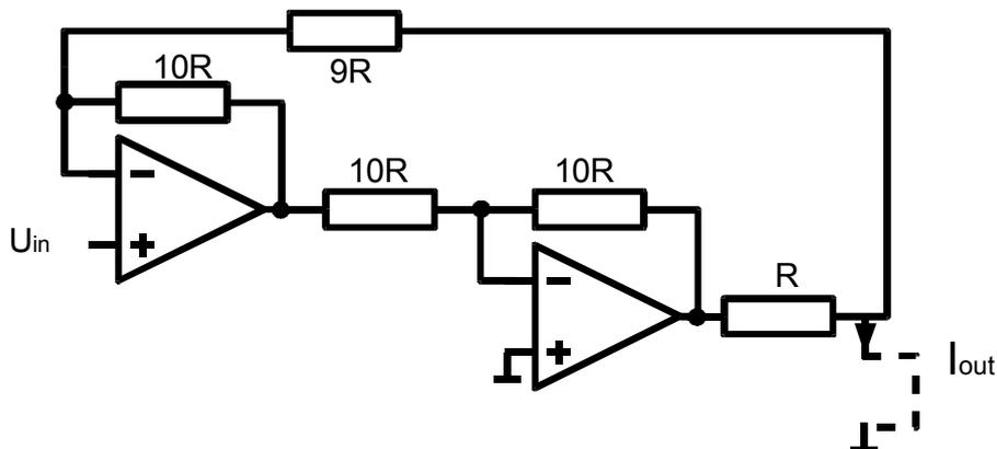
Figure 6.14 Voltage controlled current source 2
