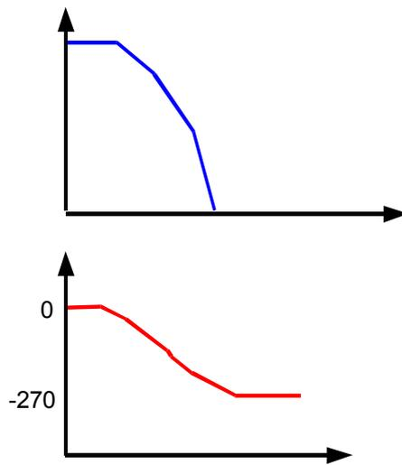
Figure 7.7 Frequency characteristics of a 3 stage amplifier
