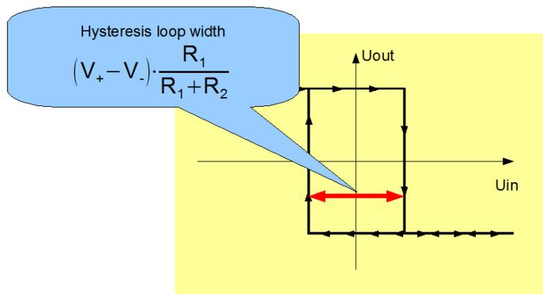
Figure 6.33 Hysteresis loop width - inverting Schmitt trigger
