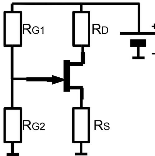
Figure 5.12 JFET polarization circuit with a voltage divider
