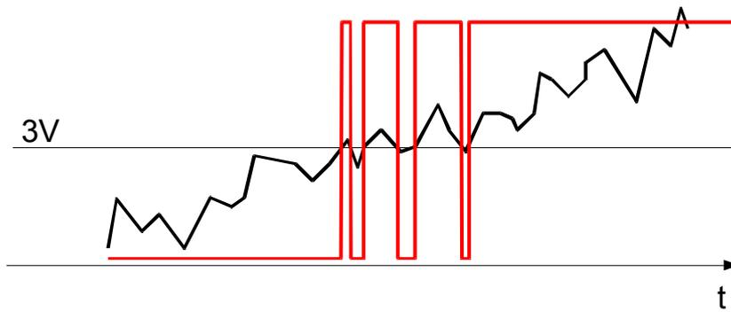
Figure 6.29 Noisy input signal (black) and comparator output (red)
