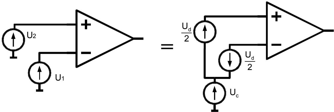
Figure 6.24 Differential and common mode voltages
