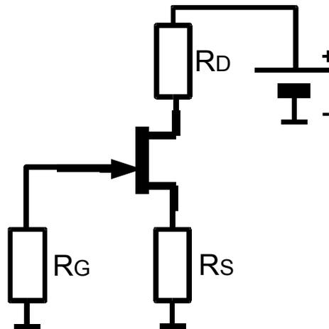
Figure 5.11 Automatic polarization circuit for JFETs - the most popular
