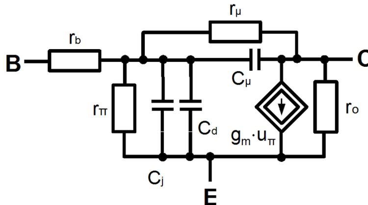
Figure 7.14 Full hybrid-pi bipolar transistor model
