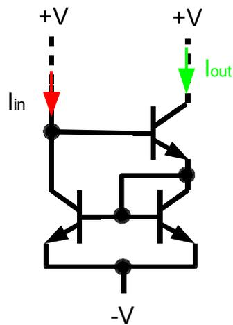
Figure 6.43 Current mirror with buffered output
