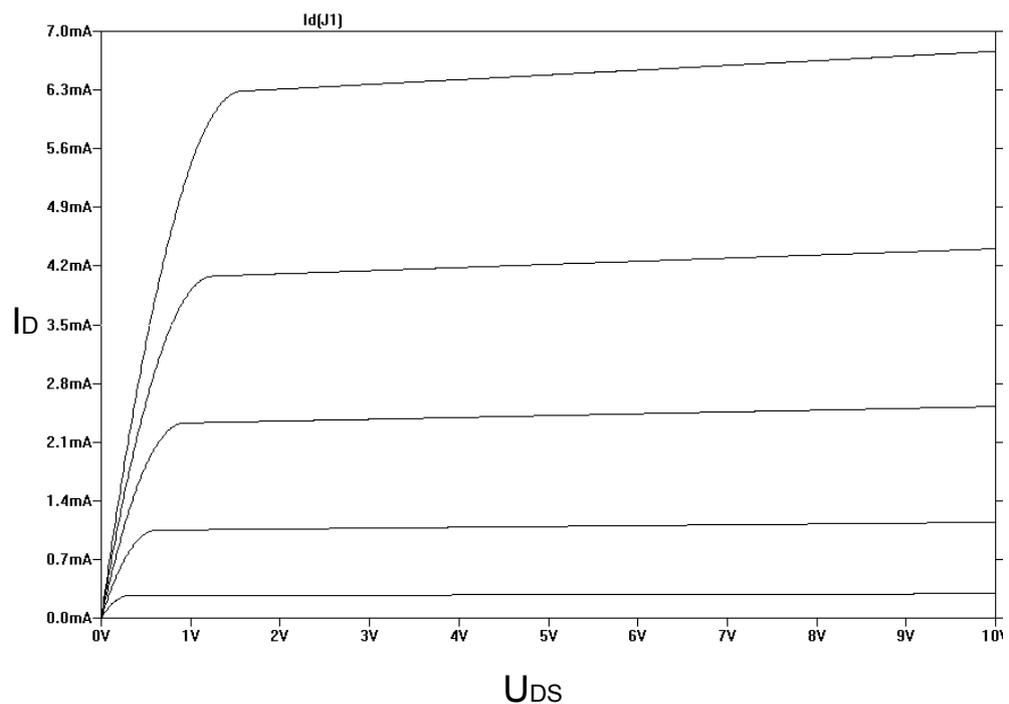
Figure 5.10 JFET transistor output characteristics
