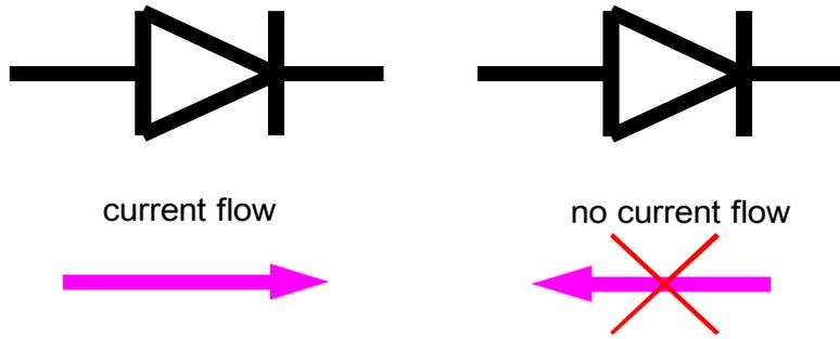
Figure 3.2 Diode current flow
