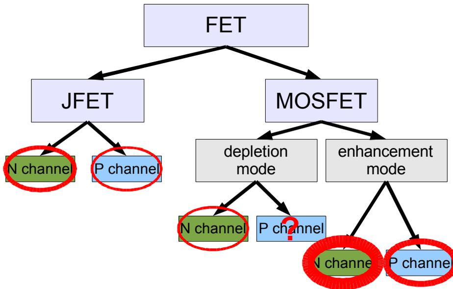
Figure 5.3 FET transistor types
