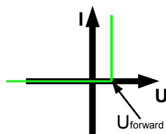
Figure 3.7 Diode model II
