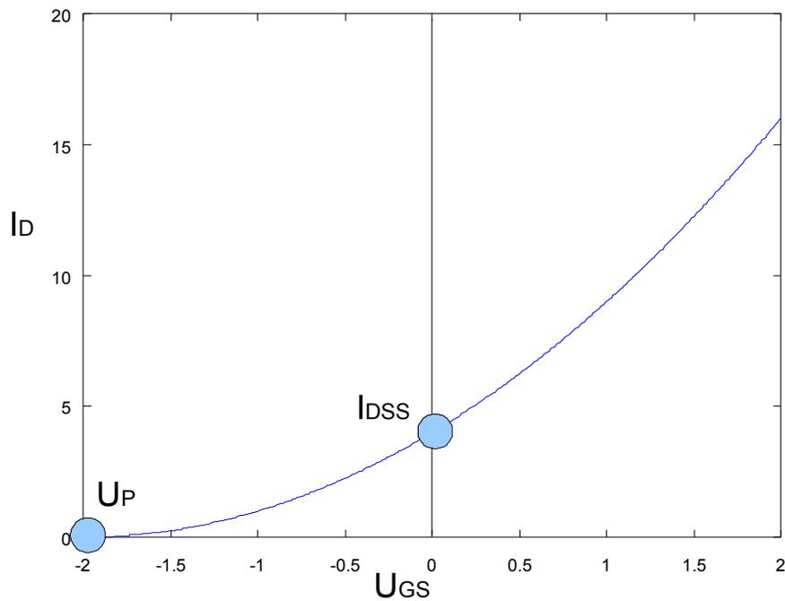
Figure 5.25 Depletion mode N channel MOSFET transfer characteristics
