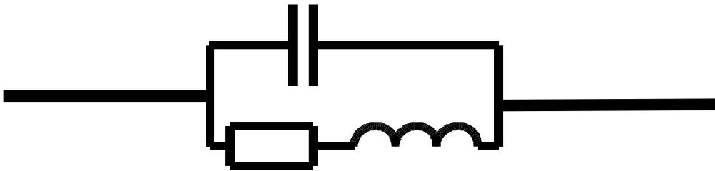
Figure 2.27 Model of parasitic elements of a real inductor
