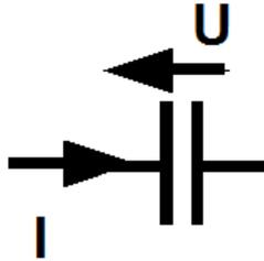
Figure 2.16 Current and voltage across a capacitor
