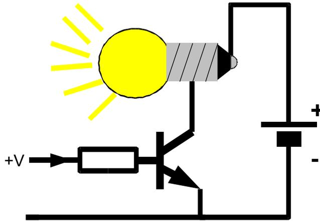
Figure 4.10 Transistor as a switch – conducting
