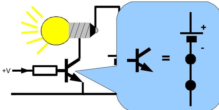
Figure 4.11 Model of a transistor in saturation
