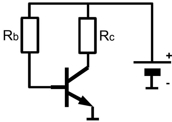
Figure 4.14 Constant base current circuit
