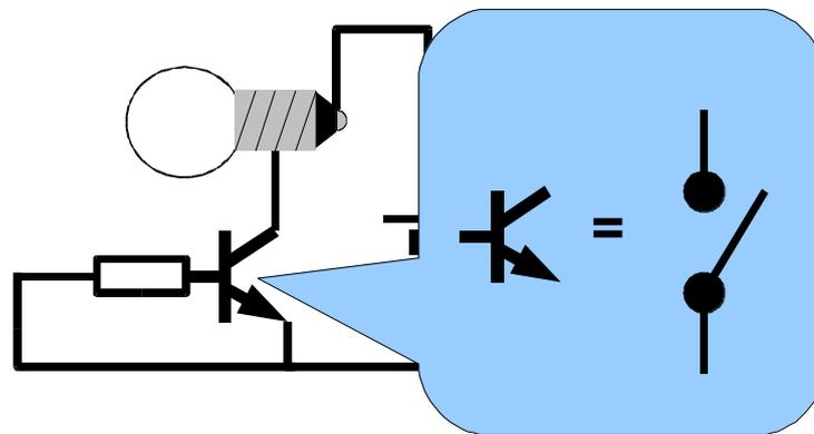
Figure 4.13 Model of a transistor in cutoff
