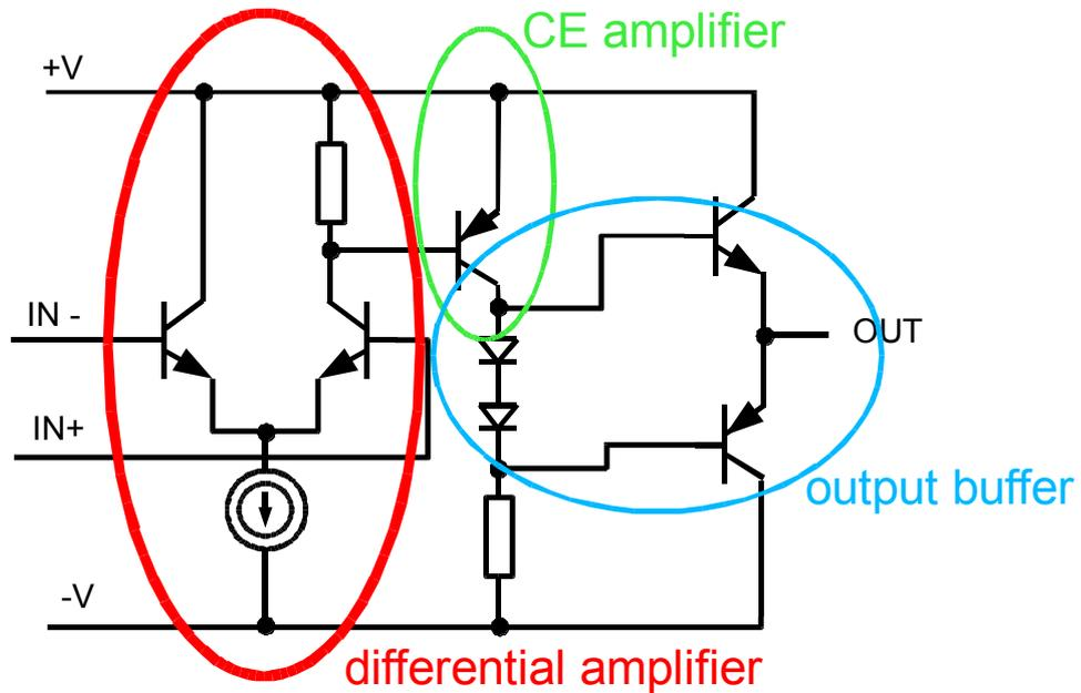
Figure 6.38 Simplified schematics of internal structure of an operational amplifier
