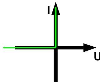
Figure 3.5 Diode model I
