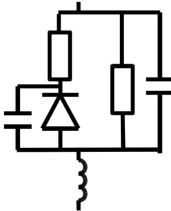
Figure 3.12 HF model of a real diode
