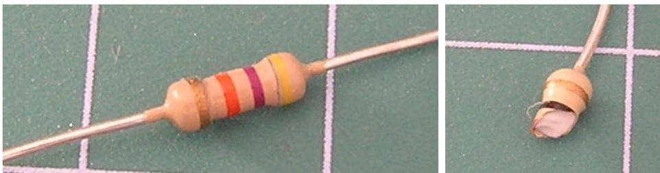
Figure 2.5 Carbon film resistor
