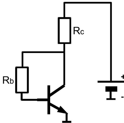
Figure 4.17 Collector feedback circuit
