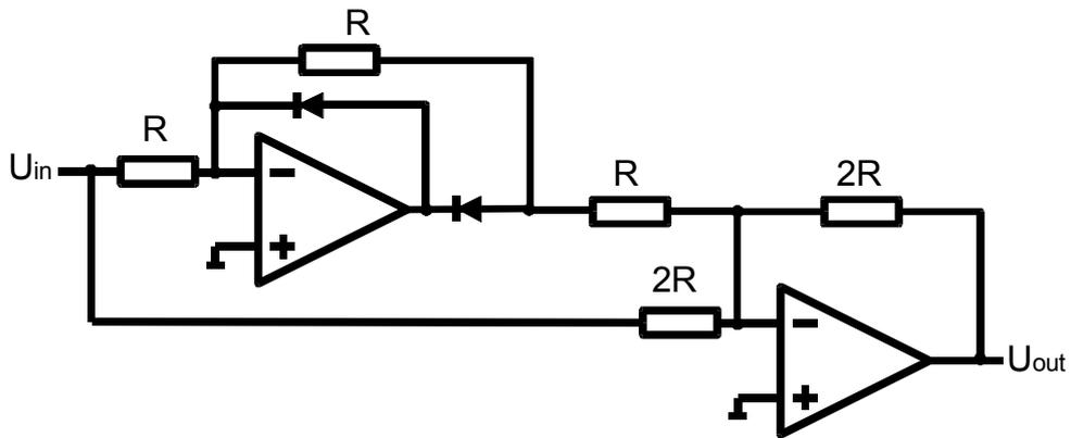
Figure 6.19 Full wave rectifier
