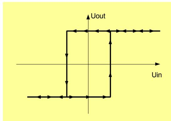
Figure 6.36 Non-inverting Schmitt trigger example operation curve
