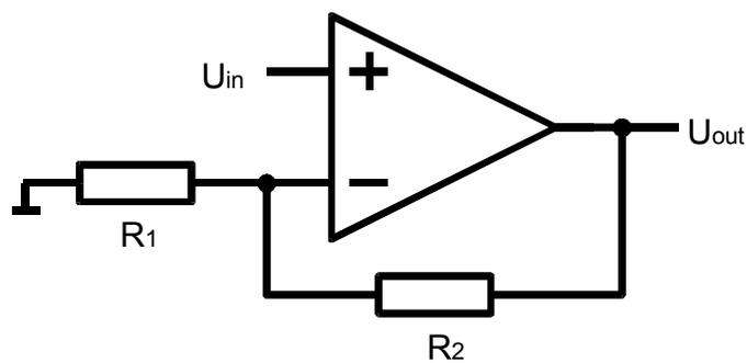
Figure 6.6 Non-inverting amplifier
