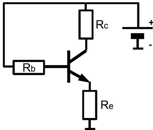
Figure 4.15 Emitter feedback circuit
