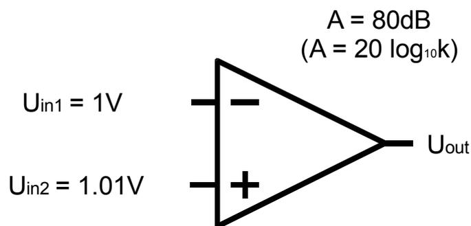
Figure 6.27 Comparator example
