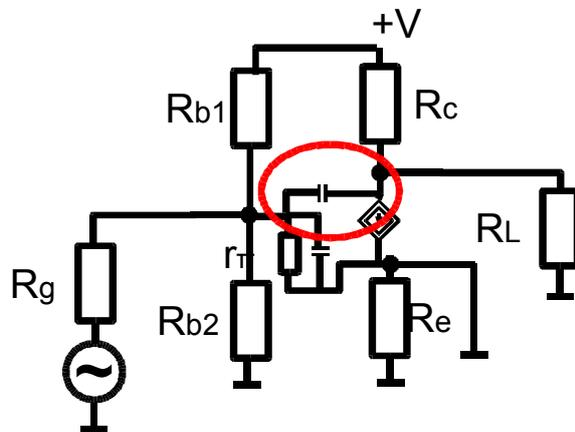
Figure 7.18 High frequency model of the transistor amplifier 3
