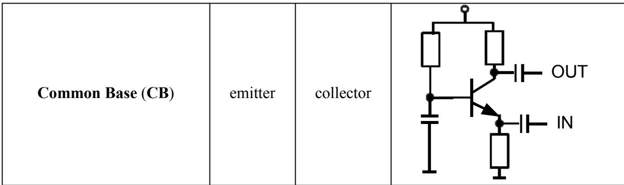
Table 4.4 Bipolar transistor amplifier typical properties depending on configuration
