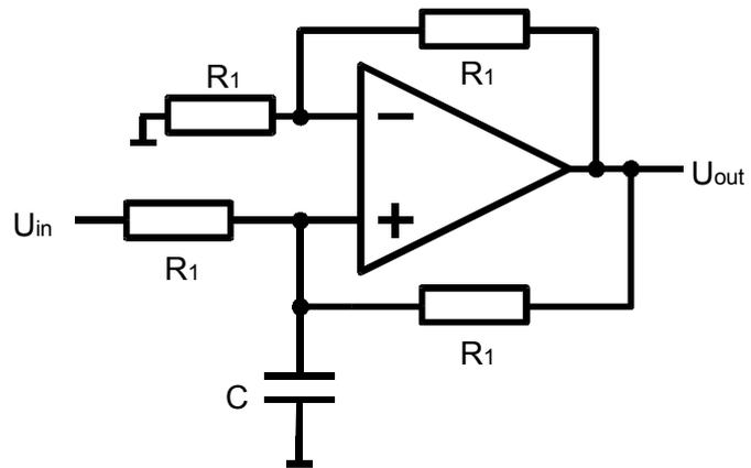
Figure 6.17 Non inverting integrator
