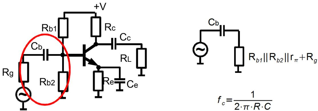
Figure 7.11 Input highpass filter
