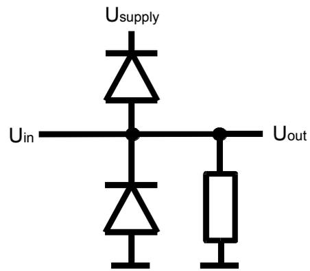
Figure 3.30 Voltage limiter
