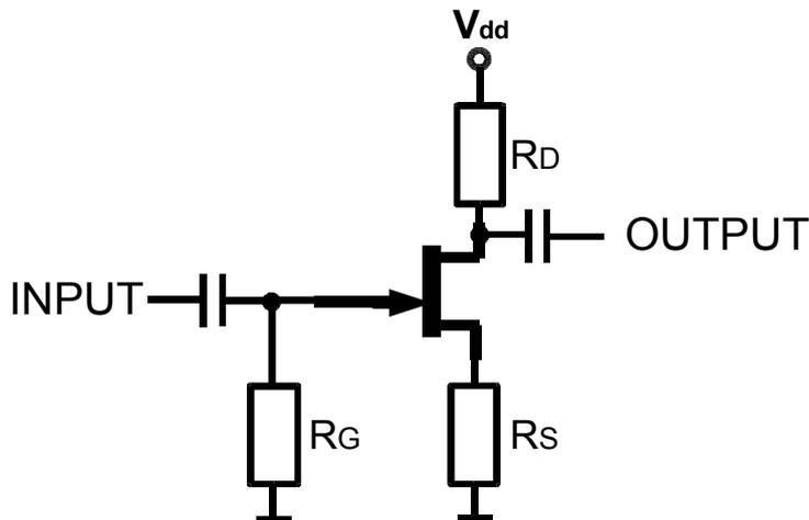
Figure 5.13 JFET transistor amplifier
