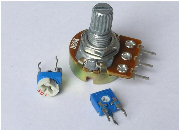
Figure 2.12 Single turn potentiometers
