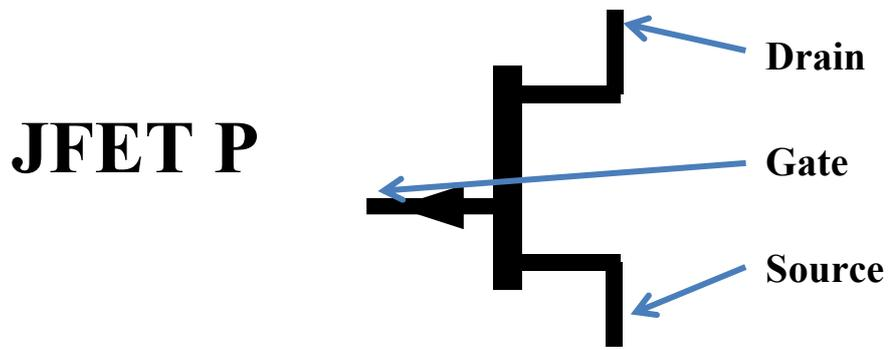
Figure 5.2 JFET-P transistor
