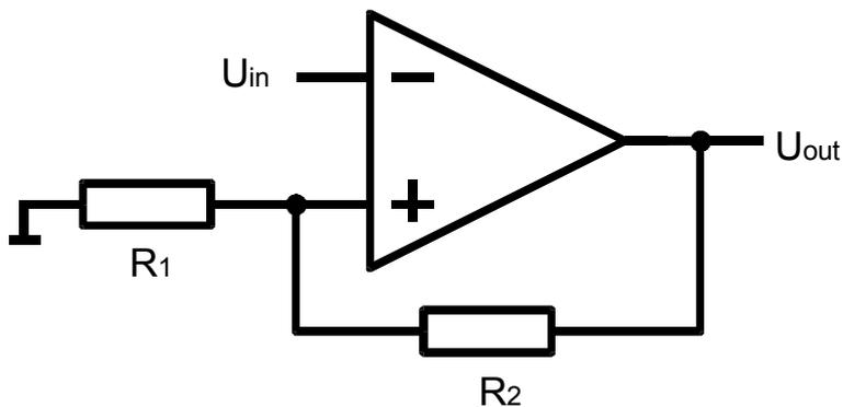
Figure 6.30 Inverting Schmitt trigger
