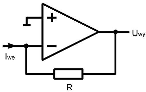
Figure 6.16 Current controlled voltage source
