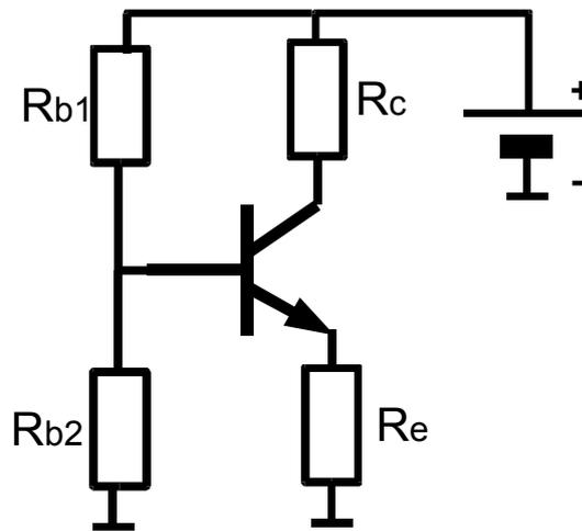
Figure 4.18 Voltage divider circuit (4 resistor circuit)
