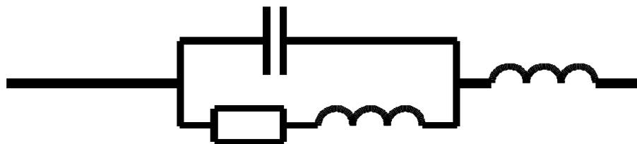
Figure 2.3 Parasitic elements of a real life resistor
