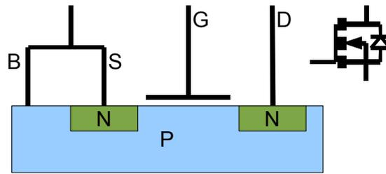
Figure 5.21 Internal structure of N channel enhancement mode MOSFET – no current flow from D to S
