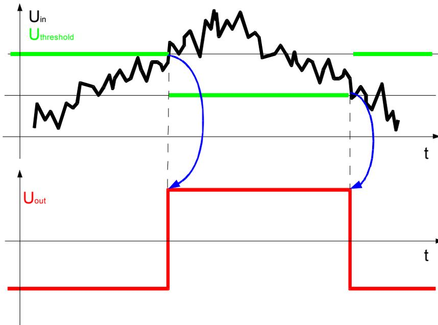
Figure 6.35 Non-inverting Schmitt trigger operation
