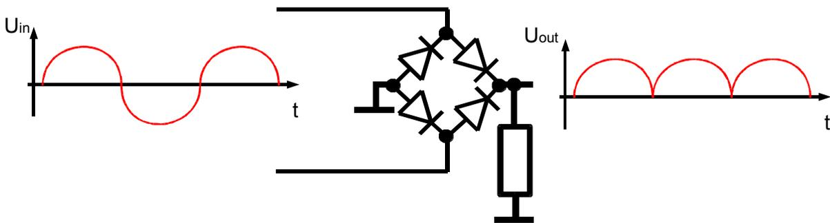
Figure 3.28 Full-wave bridge rectifier
