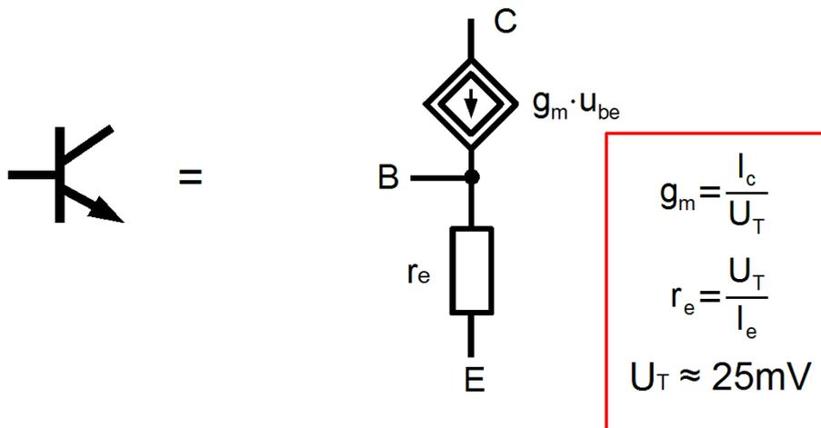
Figure 4.22 AC model of a bipolar transistor - T version
