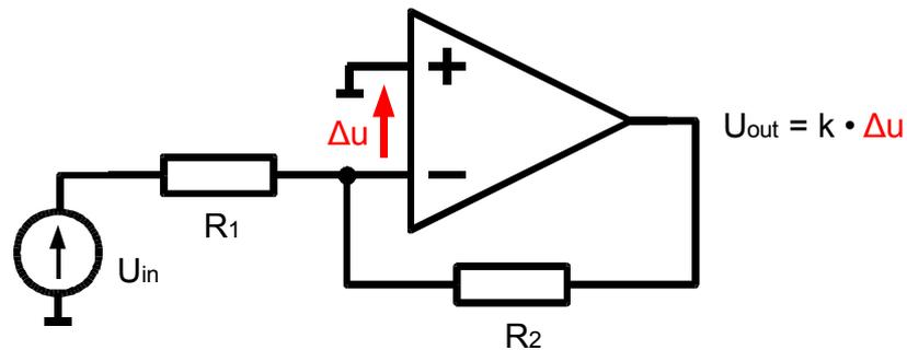
Figure 6.22 Real inverting amplifier
