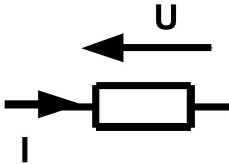
Figure 2.2. Current and voltage across the resistor
