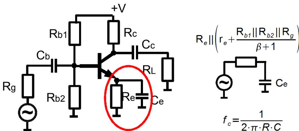
Figure 7.13 Emitter circuit frequency limit
