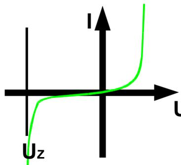
Figure 3.16 Characteristics of a Zener diode
