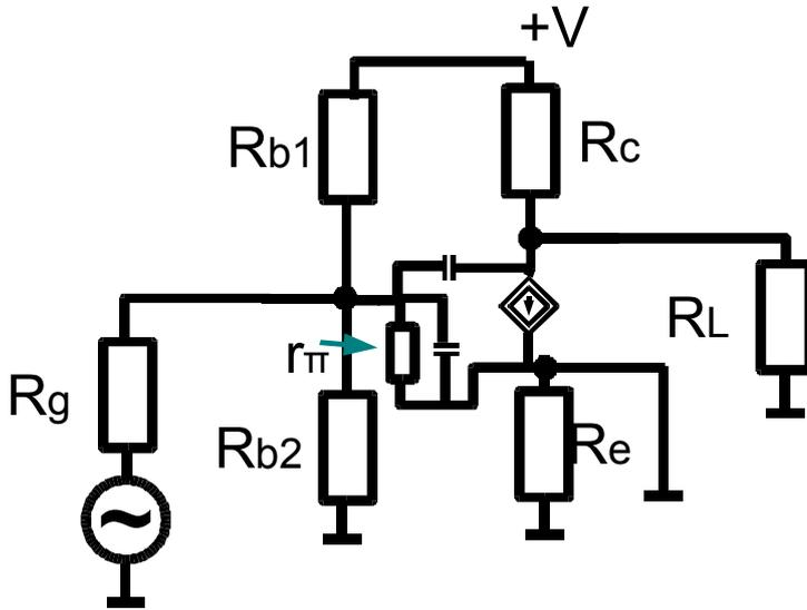
Figure 7.17 High frequency model of the transistor amplifier 2
