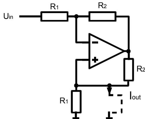
Figure 6.13 Voltage controlled current source 1
