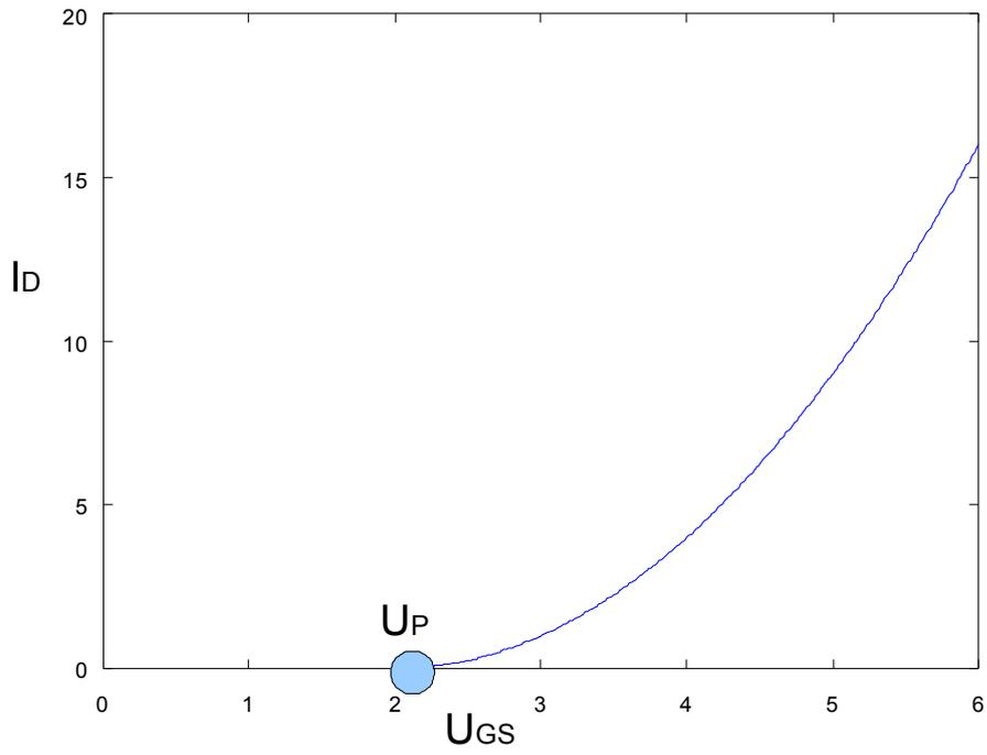
Figure 5.23 Enhancement mode N channel MOSFET transfer characteristics
