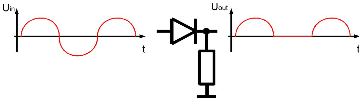
Figure 3.27 Half-wave rectifier
