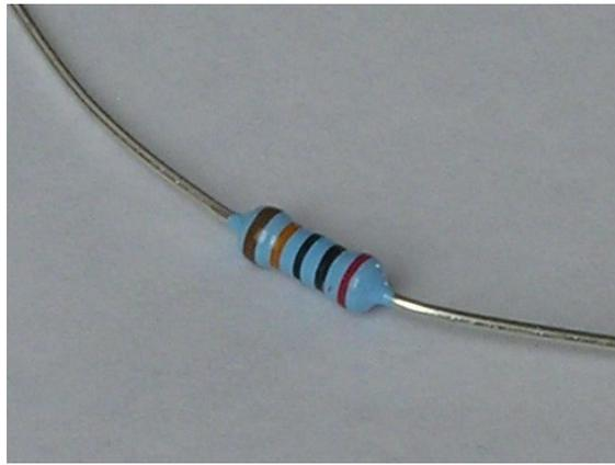
Figure 2.6 Metal film resistor
