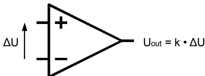
Figure 6.4 Principle of operation of an operational amplifier
