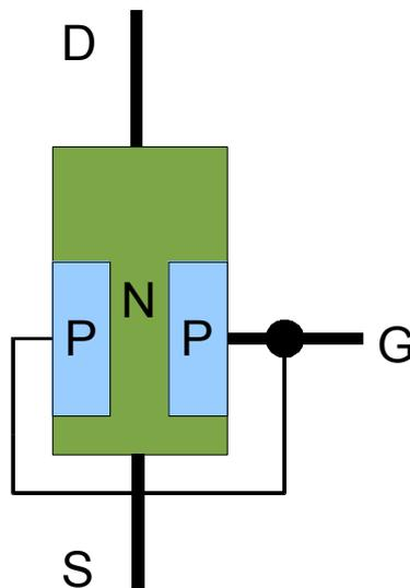
Figure 5.4 N channel JFET transistor internal structure
