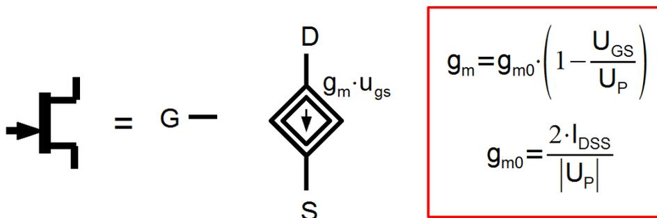
Figure 5.14 AC model of a FET transistor
