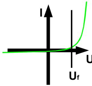
Figure 3.14 Characteristics of rectifying diode
