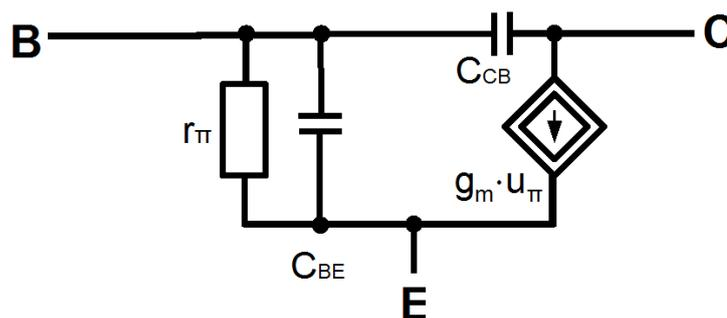
Figure 7.15 A simpler model of a transistor
