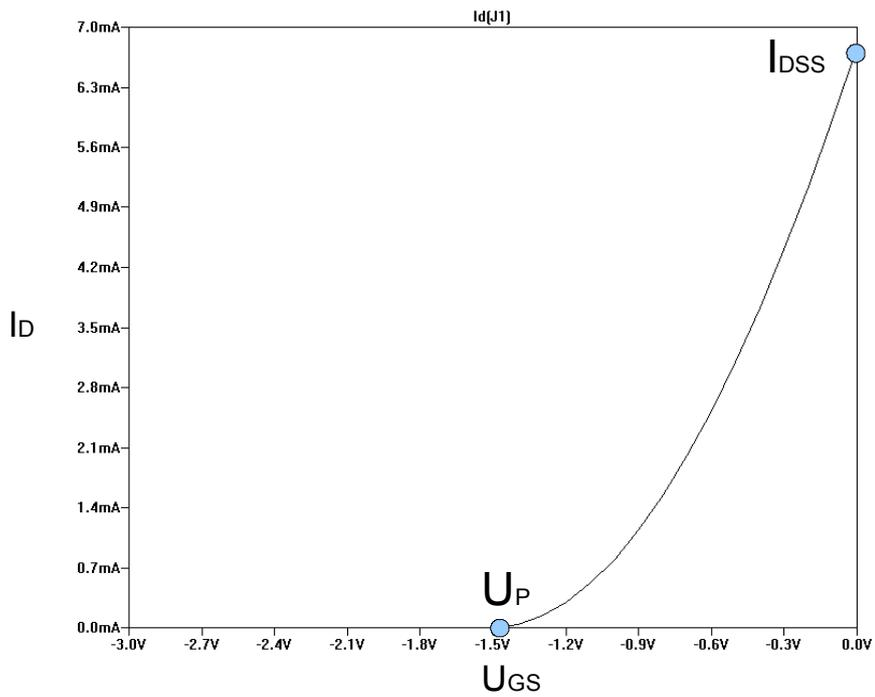
Figure 5.7 Example curve of drain current dependency on  $U_{GS}$  for JFET-N
