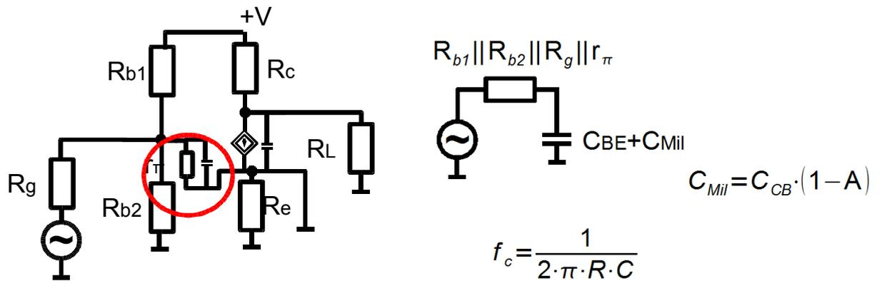
Figure 7.20 High frequency limit - base side
