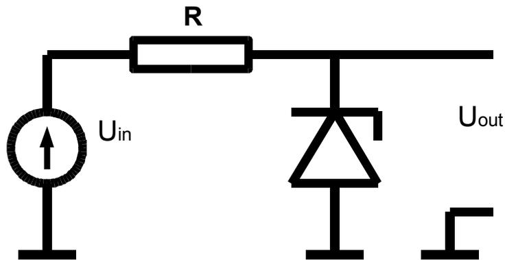
Figure 3.19 Typical application circuit of a Zener diode
