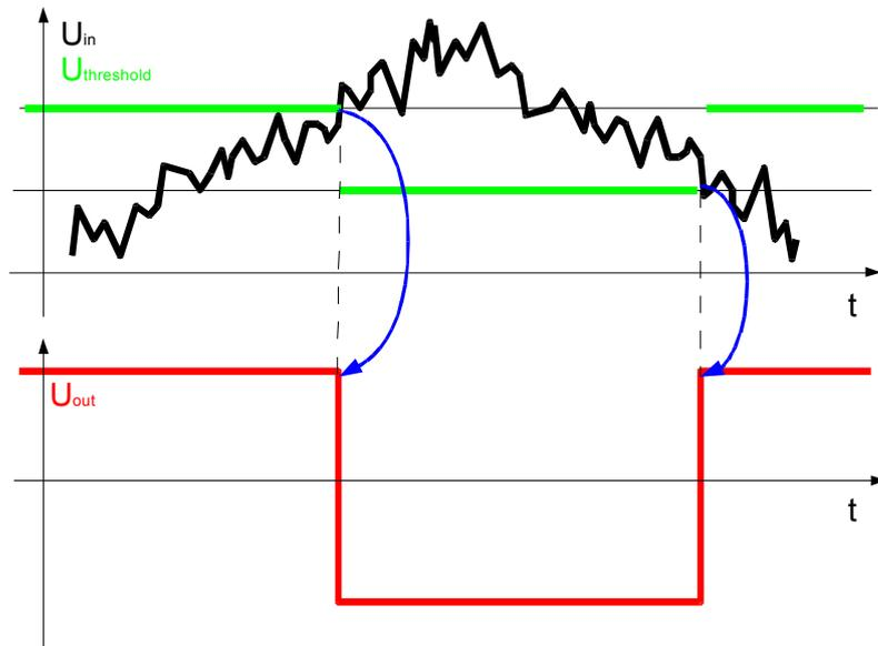
Figure 6.31 Inverting Schmitt trigger operation
