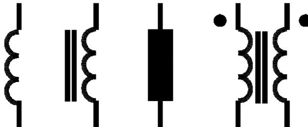
Figure 2.24 Schematic symbols for inductors. From left to right: air inductor, core inductor, alternative form of inductor marking, transformer with direction winding marks.
