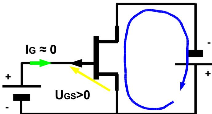
Figure 5.9 Schematical view of a typical JFET-P circuit
