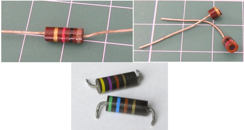
Figure 2.4 Carbon volume resistors
