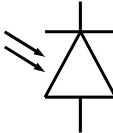
Figure 3.25 Photodiode symbol
