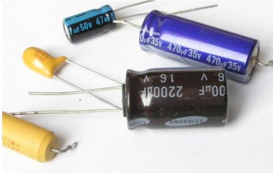
Figure 2.21 Electrolytic capacitors
