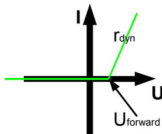
Figure 3.9 Diode model III
