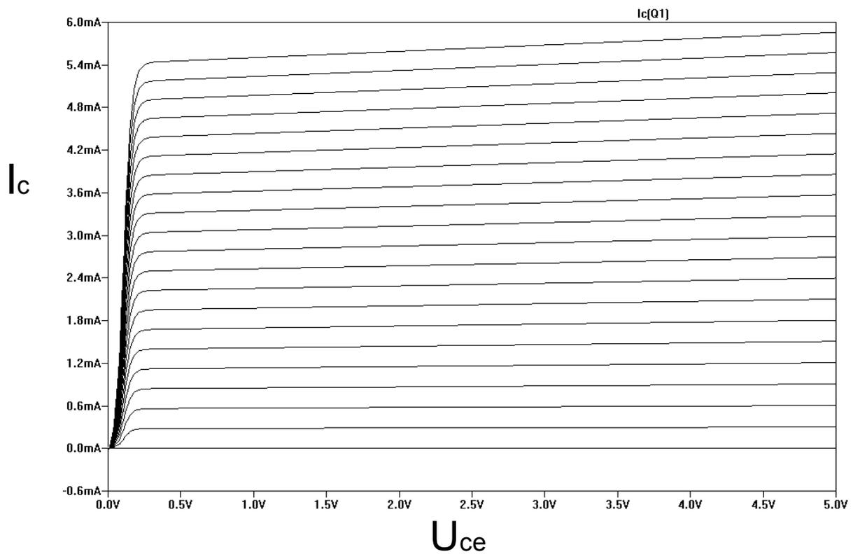
Figure 4.9 Bipolar transistor output characteristics
