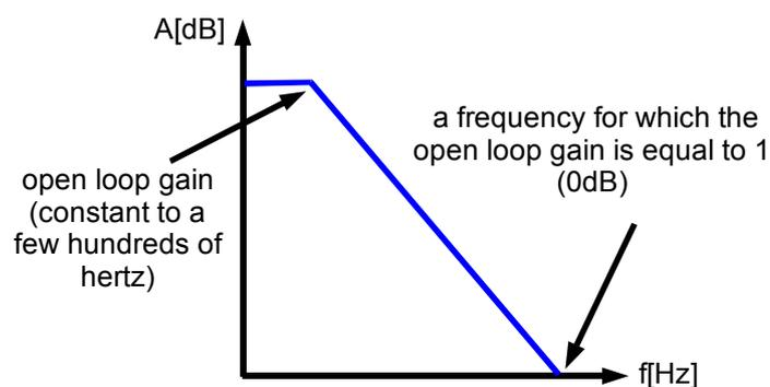
Figure 7.1 Open loop gain dependency on frequency
