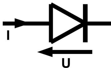
Figure 3.3 Diode voltage and current directions
