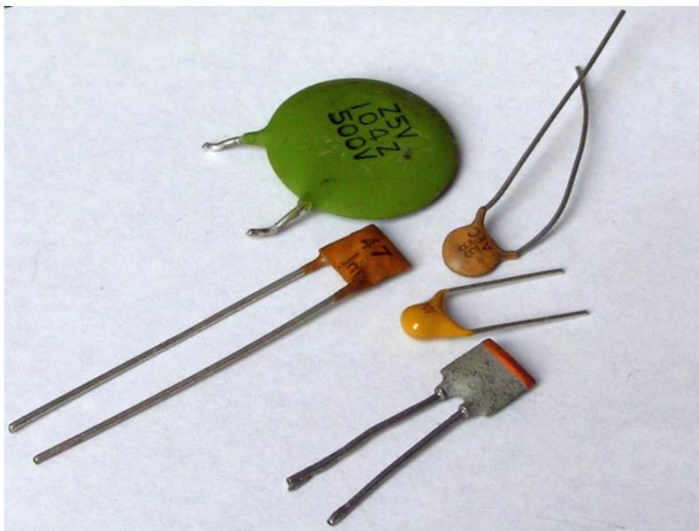
Figure 2.20 Ceramic capacitors
