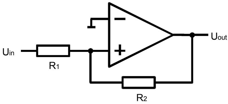
Figure 6.34 Non-inverting Schmitt trigger
