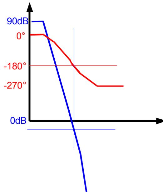
Figure 7.9 Compensated amplifier frequency response
