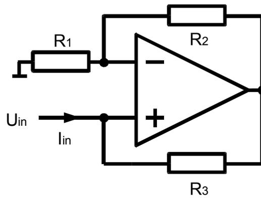
Figure 6.20 Simple impedance converter
