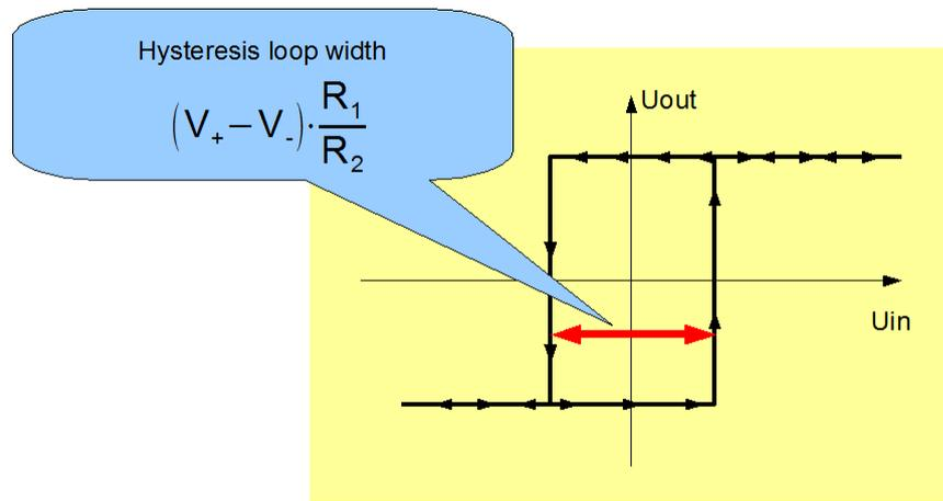
Figure 6.37 Hysteresis loop width - non-inverting Schmitt trigger
