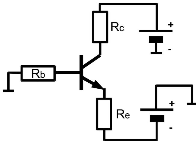
Figure 4.16 Constant emitter current circuit
