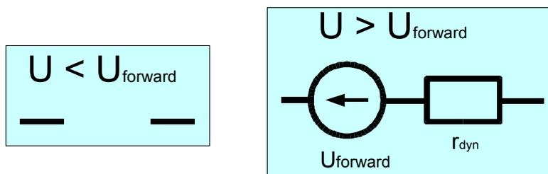
Figure 3.10 Diode equivalent circuits - model III
