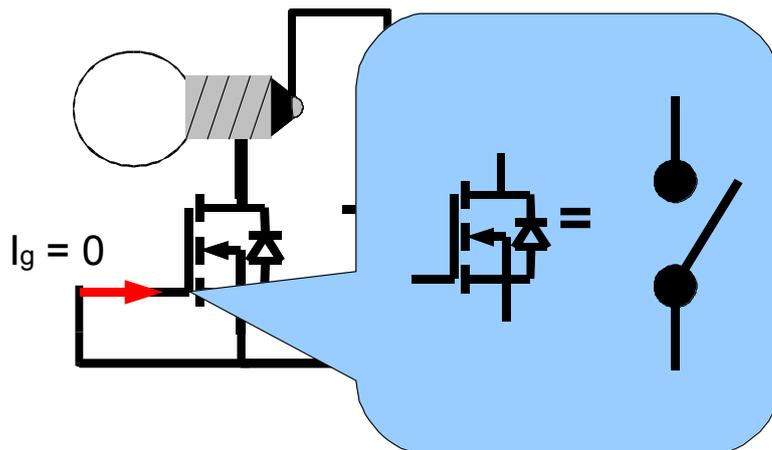
Figure 5.28 MOSFET as a switch - fully off
