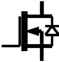
Figure 5.18 Depletion mode N channel MOSFET symbol
