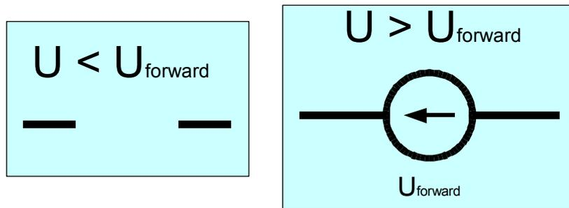
Figure 3.8 Diode equivalent circuits - model II
