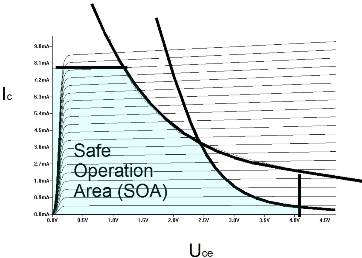
Figure 4.24 Power dissipation in bipolar transistors
