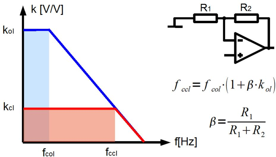
Figure 7.2 Gain-bandwidth product for an amplifier (ol = open loop, cl = closed loop)
