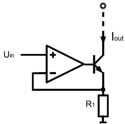
Figure 6.15 Voltage controlled current source 3
