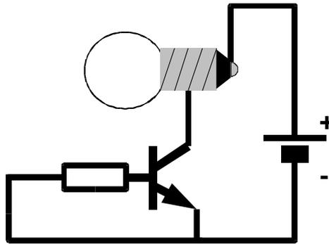
Figure 4.12 Transistor as a switch - not conducting
