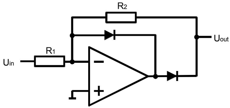
Figure 6.18 Half wave rectifier
