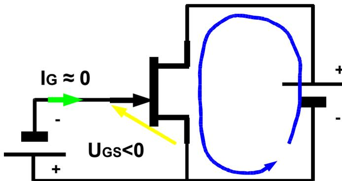
Figure 5.8 Schematical view of a typical JFET-N circuit
