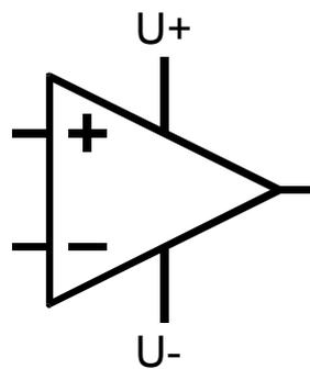
Figure 6.3 Operational amplifier with power supply pins visible
