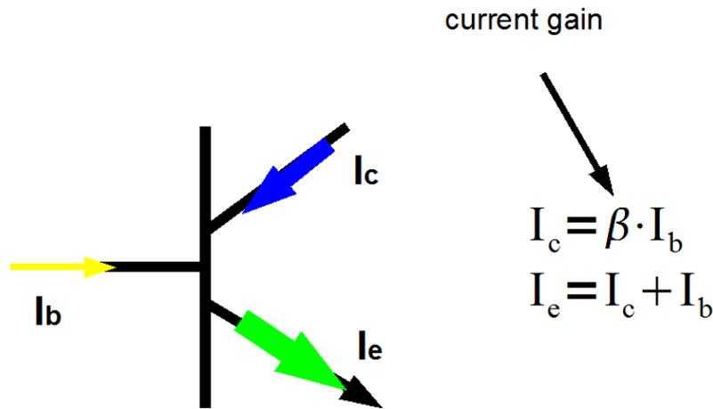
Figure 4.5 Currents in NPN transistor
