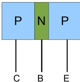
Figure 4.4 Internal structure of PNP transistor
