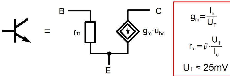
Figure 4.21 AC model of bipolar transistor - PI version
