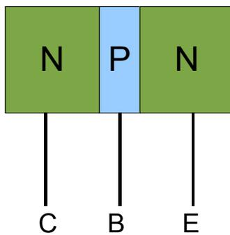
Figure 4.3 Internal structure of NPN transistor
