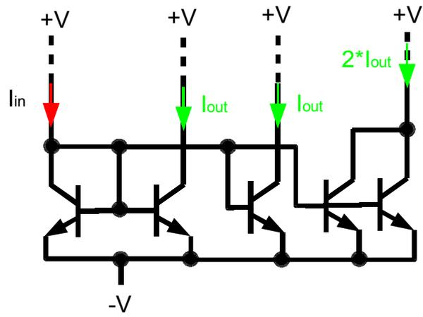
Figure 6.41 Multiple output current mirror
