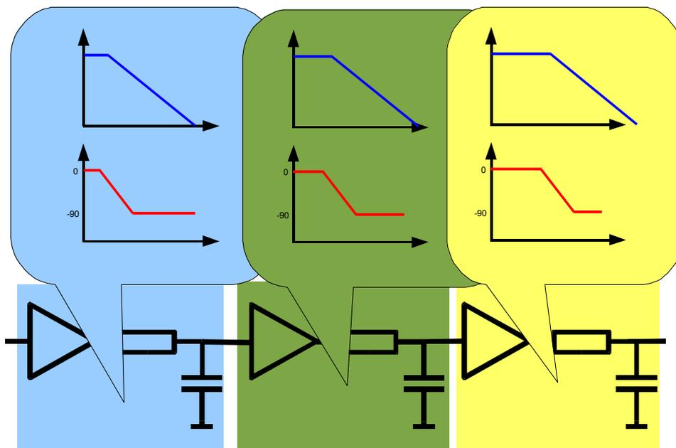
Figure 7.5 Multi stage amplifier frequency characteristics
