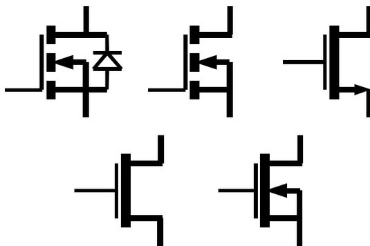
Figure 5.19 Different symbols used for N channel enhancement mode MOSFET
