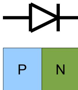
Figure 3.4 Semiconductor types in a diode
