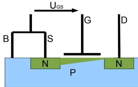
Figure 5.22 Internal structure of N channel enhancement mode MOSFET – current can flow from D to S through the induced channel
