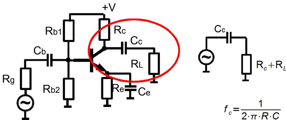
Figure 7.12 Output highpass filter
