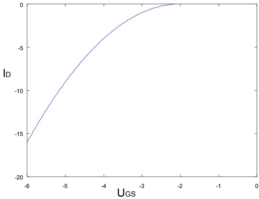
Figure 5.24 Enhancement mode P channel MOSFET transfer characteristics
