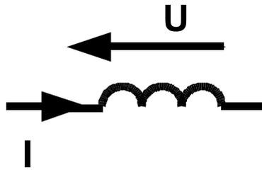
Figure 2.25 Current and voltage across an inductor
