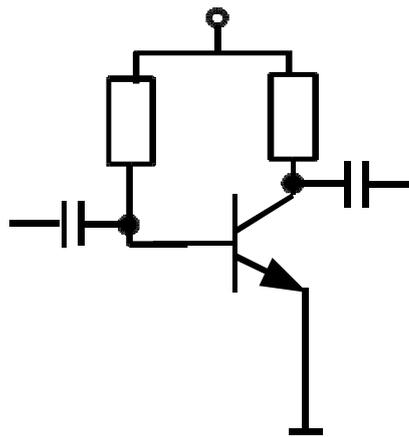
Figure 4.20 Example circuit for DC analysis of a transistor amplifier
