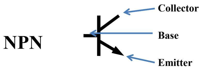
Figure 4.1 NPN transistor symbol
