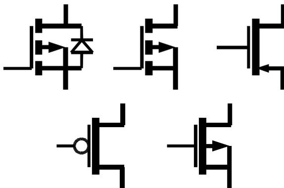
Figure 5.20 Different symbols used for P channel enhancement mode MOSFET
